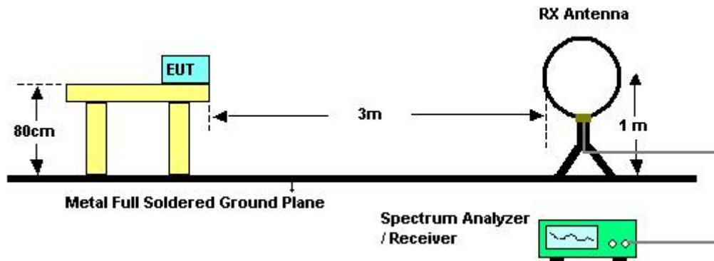
For Radiated Emissions: 30MHz~1GHz
