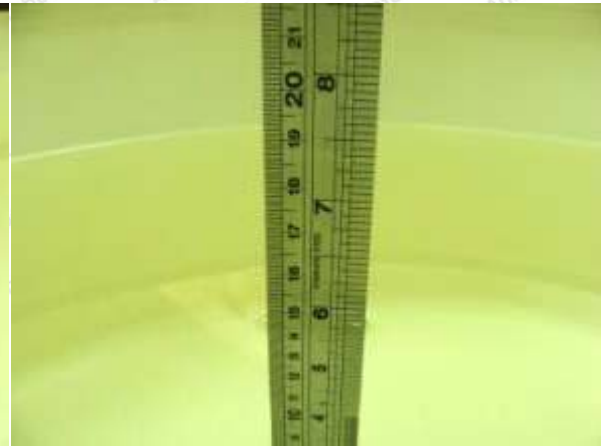
Photo of Liquid Height for Body SAR
