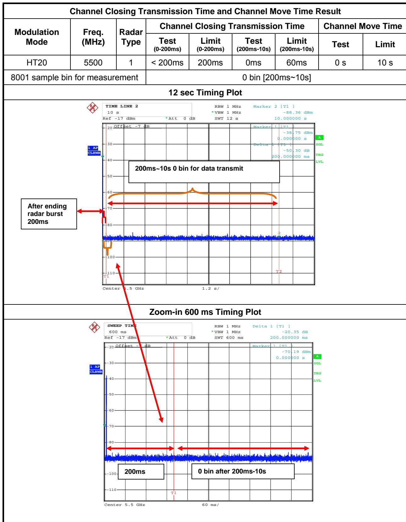
**Channel Closing Transmission Time and Channel Move Time Result**
