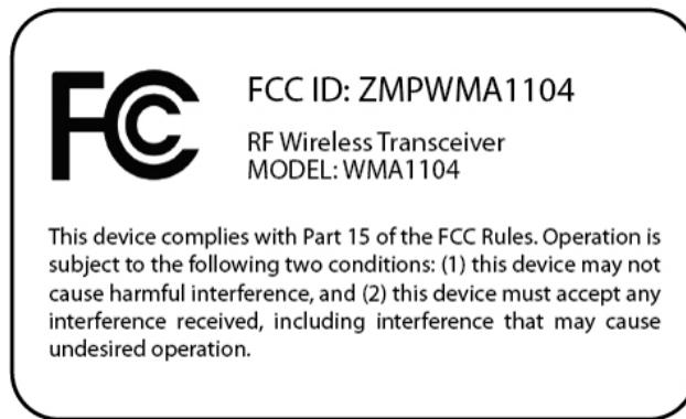
**Specifications:** Text is Black in color and justified. Labels are printed in indelible ink on permanent adhesive or silk-screened onto the EUT or shall be affixed at a conspicuous location on the EUT.
