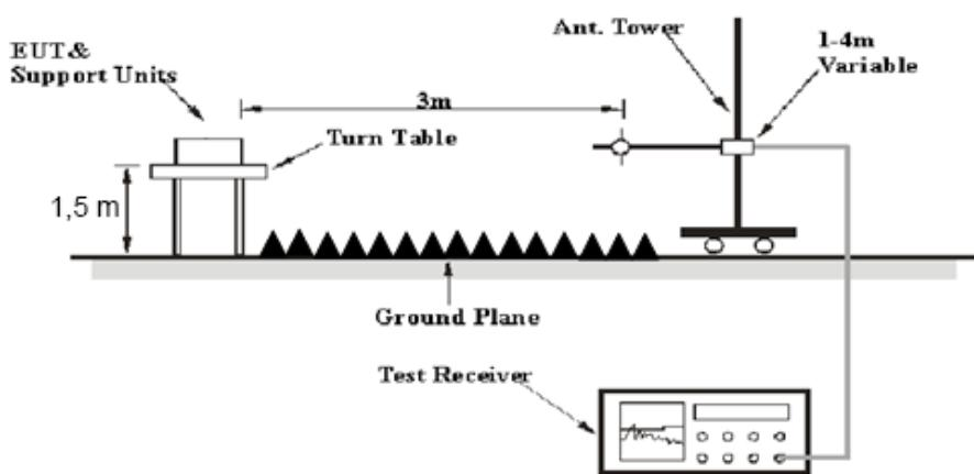
The radiated emission below 1GHz tests were performed in the 3 meters chamber test site A, above 1GHz tests were performed in the 3 meters chamber test site B, using the setup accordance with the ANSI C63.10-2013. The specification used was the FCC 15.209, and FCC 15.247 limits.
