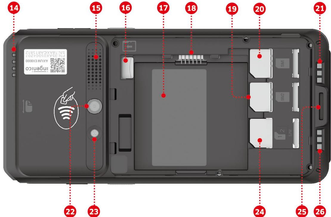
14. LEDs for Contactless Card
