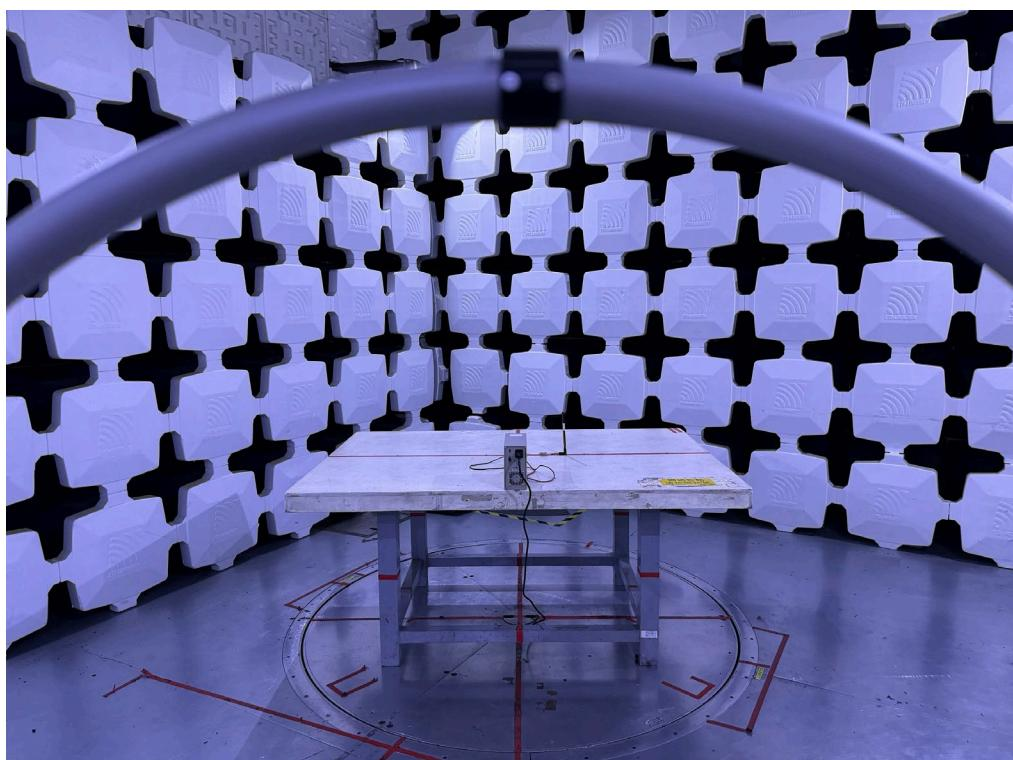
**Radiated Emissions Test Photos****30 MHz to 1000 MHz**
