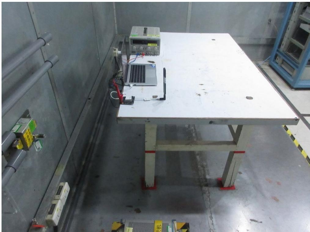
**Radiated Emissions Test Photos****9 kHz to 30 MHz**
