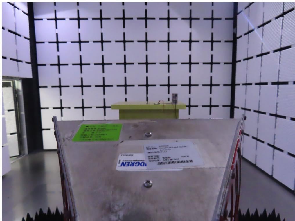
**Radiated Emissions Test Photos****Harmonic (18 GHz to 26.5 GHz)**
