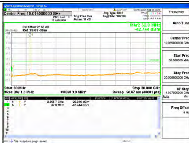
B7-30M-20G / 15MHz / High CH / QPSK
