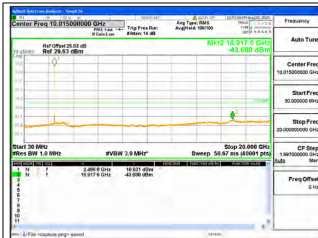
B41-30M-20G / 15MHz / Low CH / QPSK
