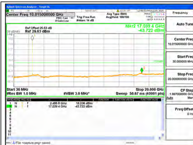
B41-30M-20G / 5MHz / Low CH / QPSK
