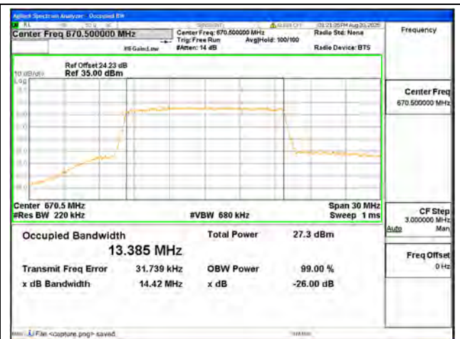
B71 / 15MHz / 16QAM/ Low CH
