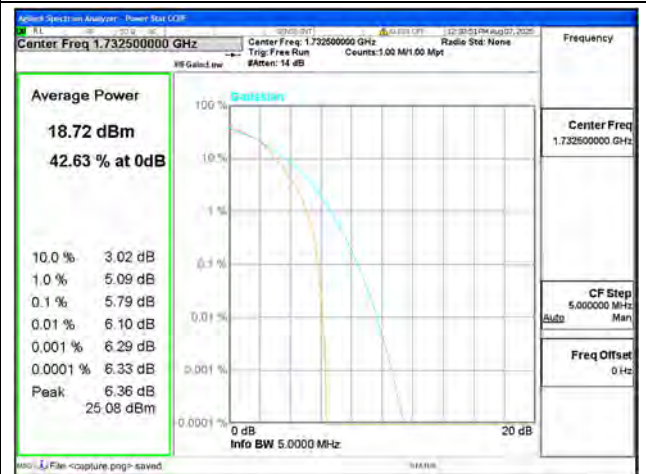
B4 / 1.4MHz / Mid CH / 16QAM
