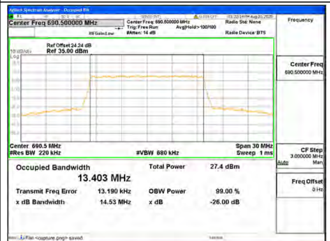
B71 / 15MHz / 16QAM/ High CH
