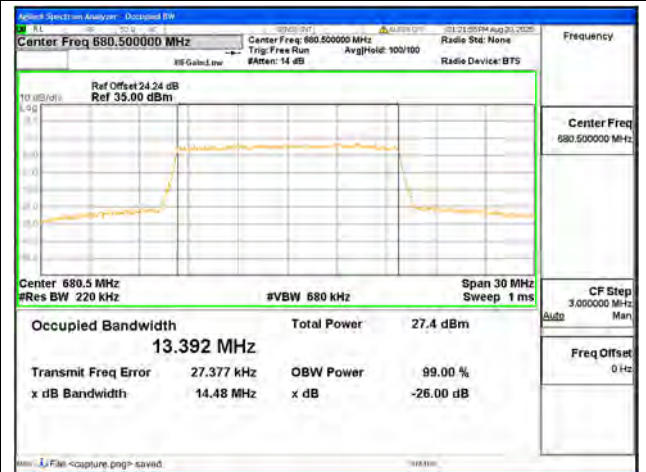
B71 / 15MHz / 16QAM/ Mid CH
