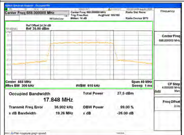
B71 / 20MHz / 16QAM/ High CH
