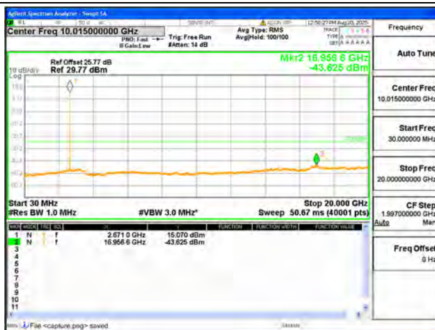
B41-30M-20G / 20MHz / High CH / QPSK
