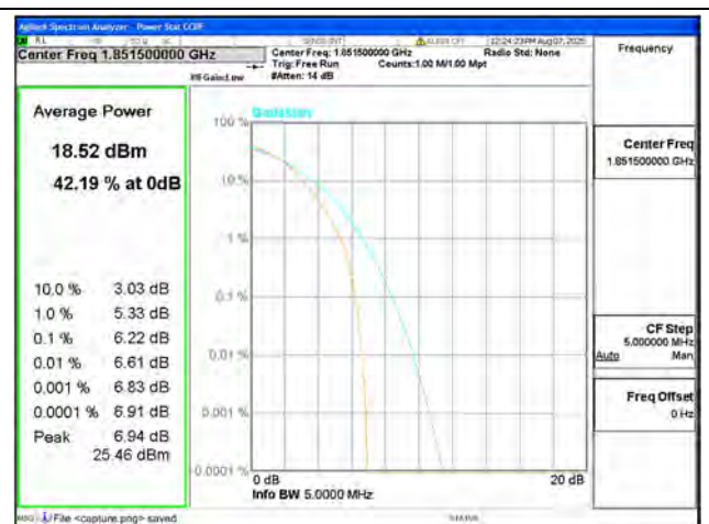
B2 / 3MHz / Low CH / 16QAM
