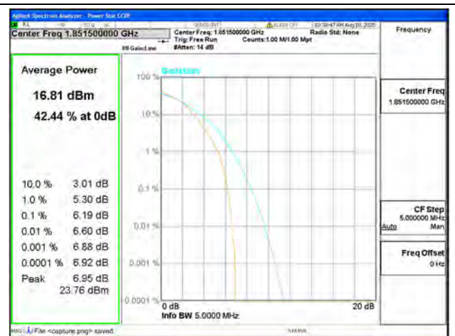
B25 / 3MHz / Low CH / 16QAM
