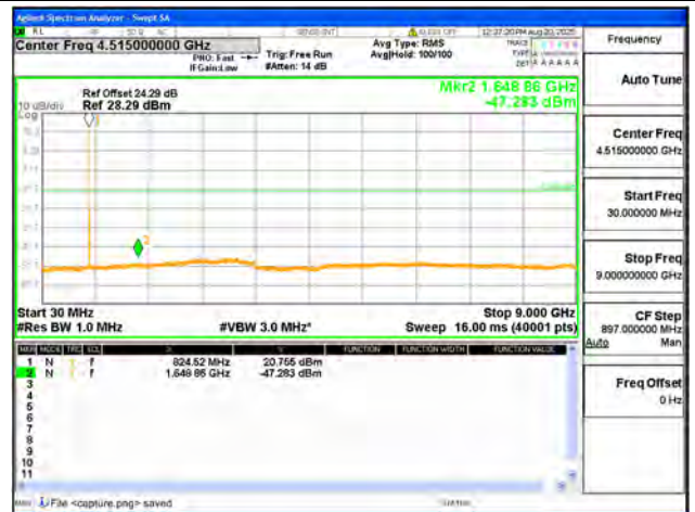
B26 Part22 / 3MHz / Low CH / QPSK
