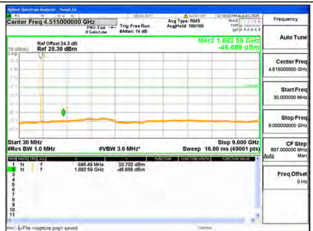
B26 Part22 / 3MHz / High CH / QPSK
