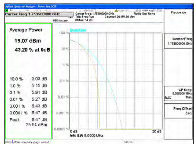
B4 / 3MHz / High CH / 16QAM
