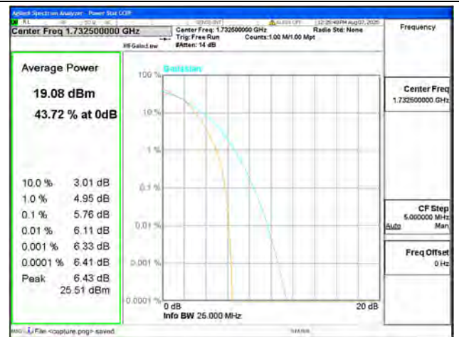
B4 / 15MHz / Mid CH / 16QAM
