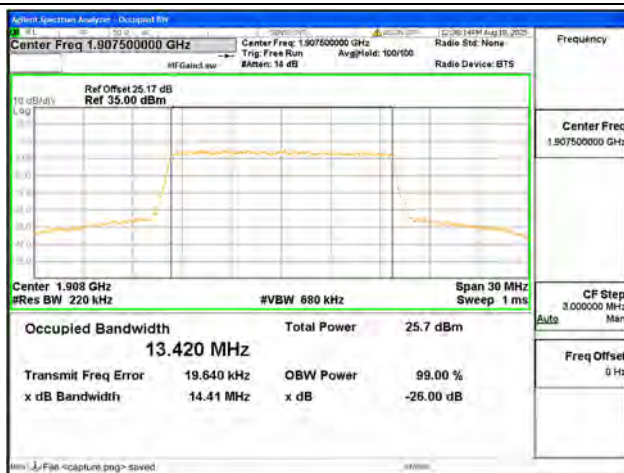
B25 / 15MHz / QPSK/ High CH
