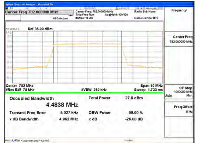
B13 / 5MHz / 16QAM/ Mid CH
