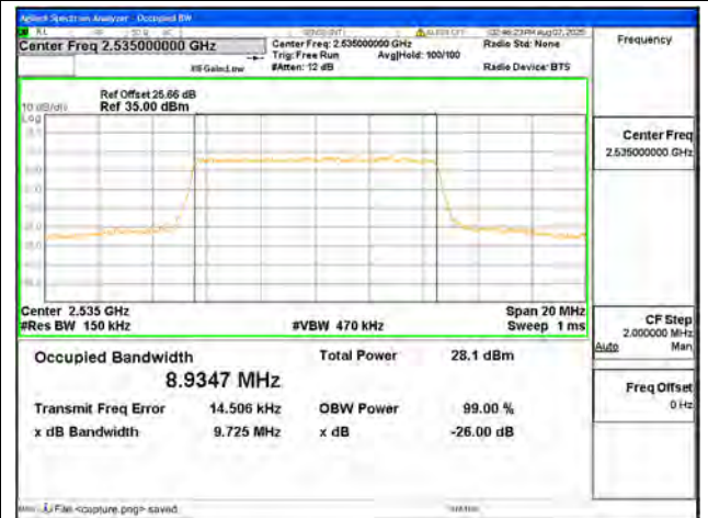
B7 / 10MHz / 16QAM/ Mid CH
