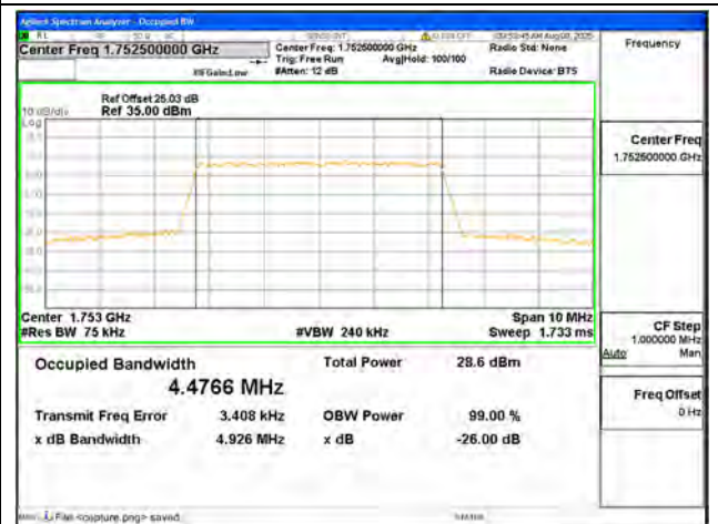
B4 / 5MHz / 16QAM/ High CH
