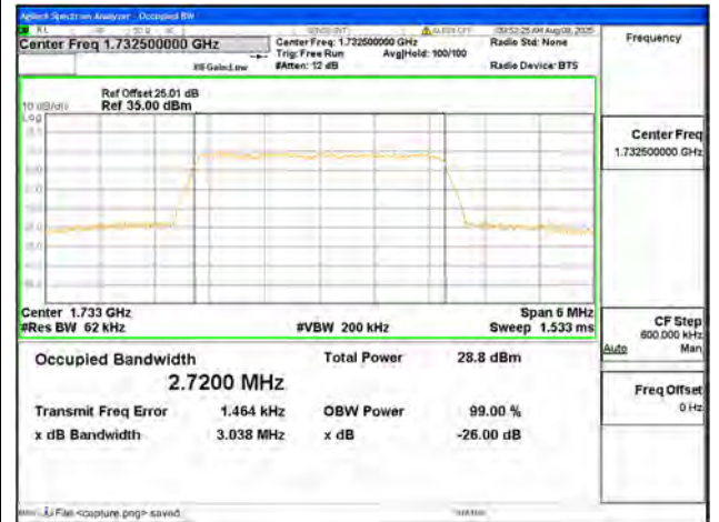
B4 / 3MHz / 16QAM/ Mid CH
