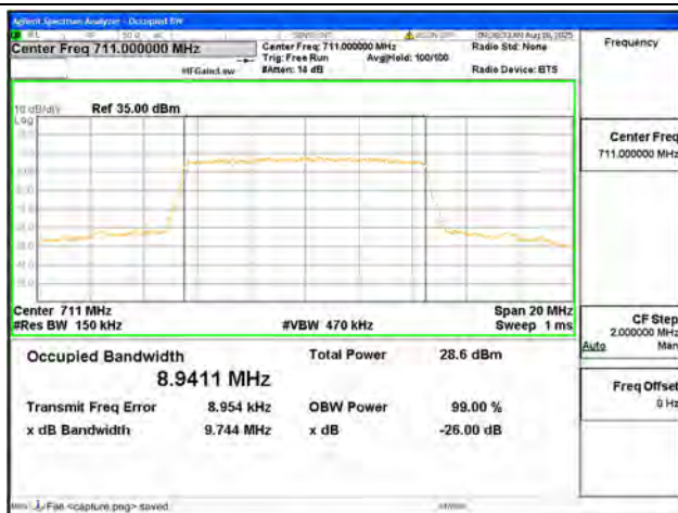
B12 / 10MHz / QPSK/ High CH
