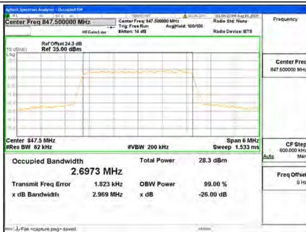
B26 Part22 / 3MHz / QPSK/ High CH
