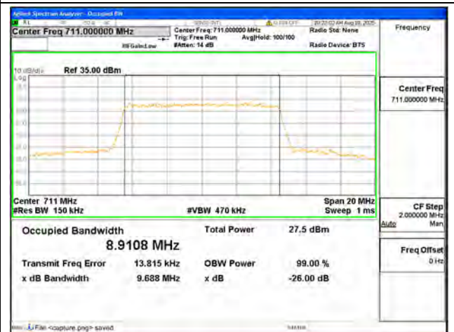
B17 / 10MHz / 16QAM/ High CH
