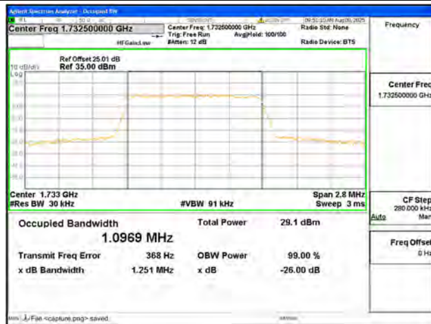
B4 / 1.4MHz / QPSK/ Mid CH
