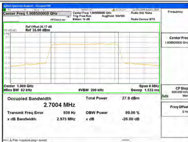
B2 / 3MHz / QPSK/ High CH
