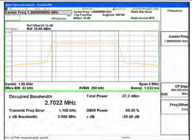
B2 / 3MHz / 16QAM/ Mid CH
