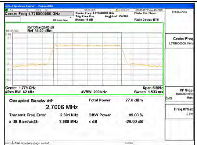
B66 / 3MHz / 16QAM/ High CH
