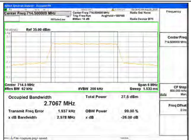
B12 / 3MHz / 16QAM/ High CH
