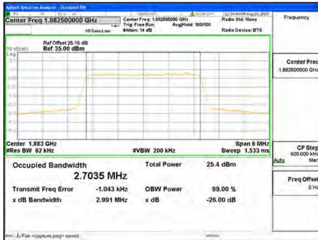
B25 / 3MHz / QPSK/ Mid CH
