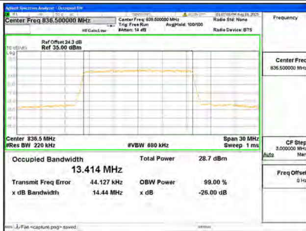
B26 Part22 / 15MHz / QPSK/ Mid CH
