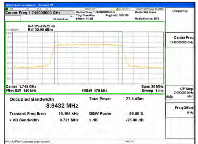
B66 / 10MHz / 16QAM/ Mid CH
