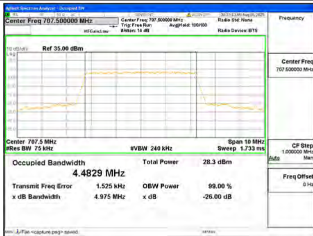
B12 / 5MHz / QPSK/ Mid CH
