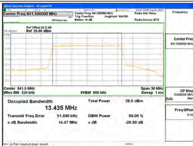
B26 Part22 / 15MHz / QPSK/ High CH
