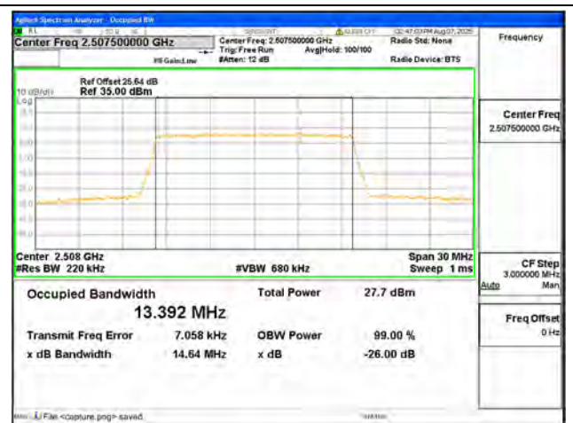
B7 / 15MHz / 16QAM/ Low CH
