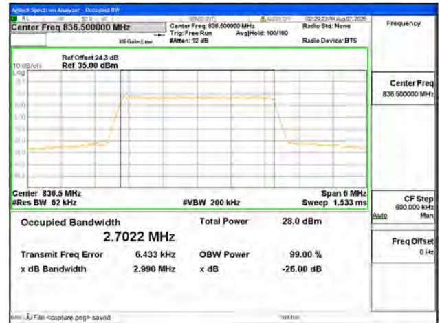
B5 / 3MHz / 16QAM/ Mid CH
