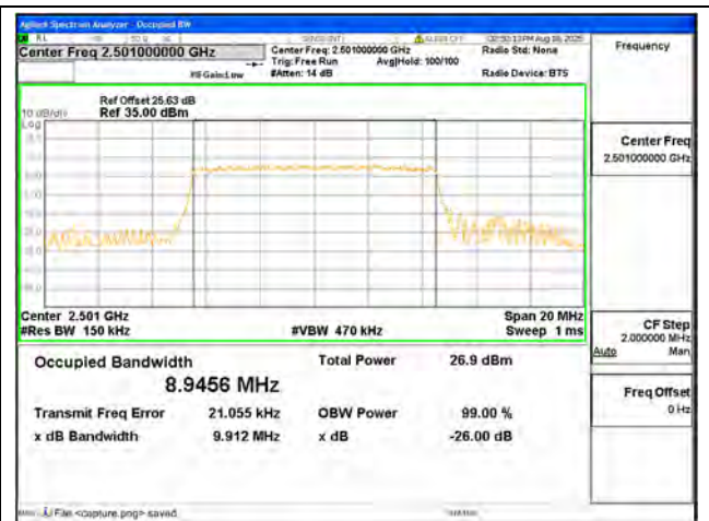
B41 / 10MHz / 16QAM/ Low CH
