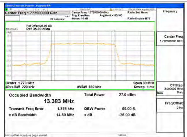
B66 / 15MHz / 16QAM/ High CH
