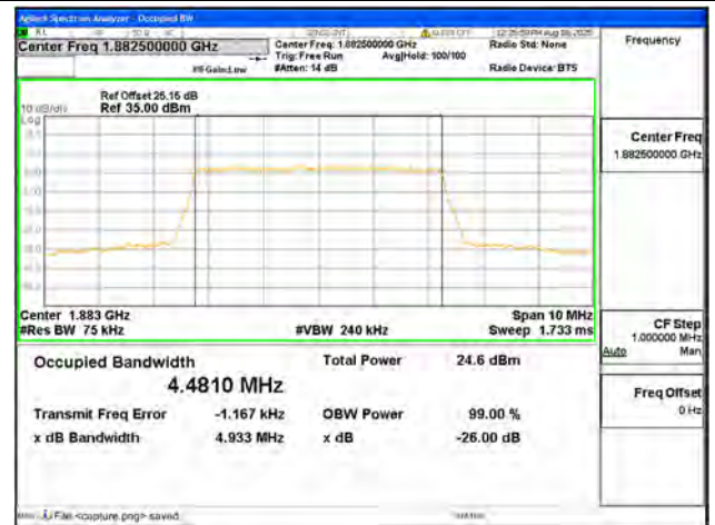
B25 / 5MHz / 16QAM/ Mid CH
