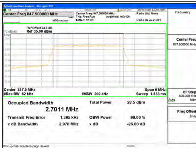
B5 / 3MHz / QPSK/ High CH
