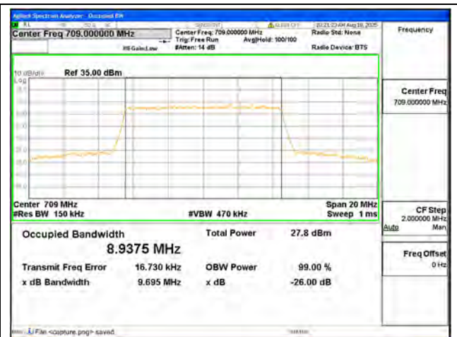
B17 / 10MHz / 16QAM/ Low CH
