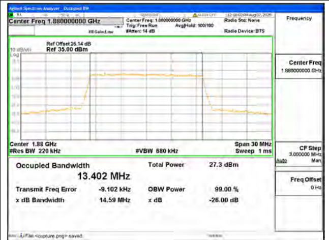
B2 / 15MHz / 16QAM/ Mid CH
