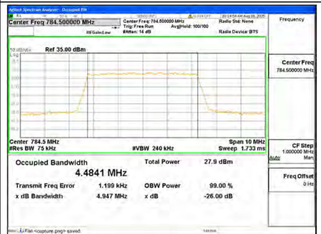
B13 / 5MHz / 16QAM/ High CH
