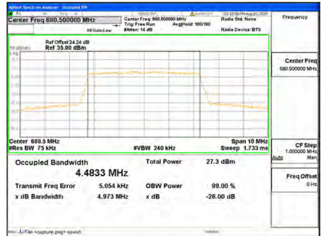
B71 / 5MHz / 16QAM/ Mid CH
