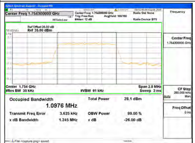
B4 / 1.4MHz / 16QAM/ High CH
