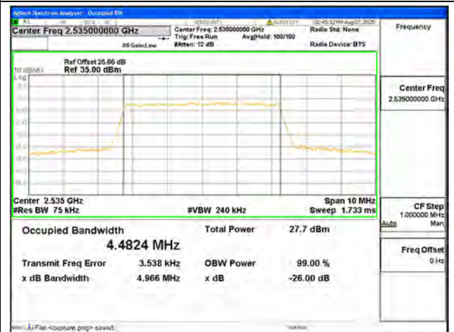
B7 / 5MHz / 16QAM/ Mid CH
