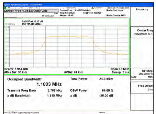
B25 / 1.4MHz / 16QAM/ High CH
