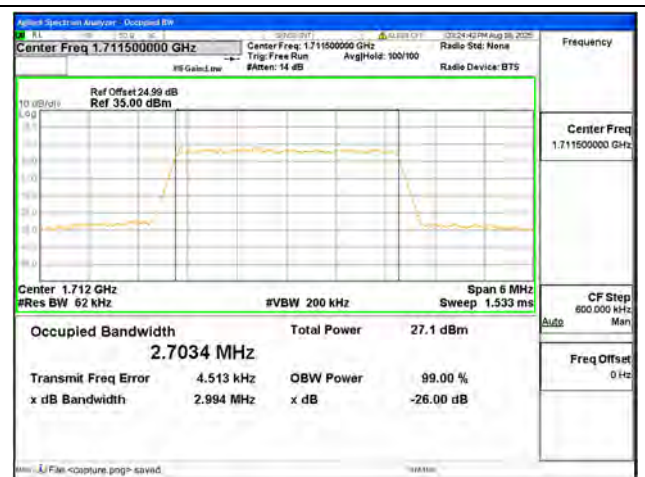
B66 / 3MHz / 16QAM/ Low CH
