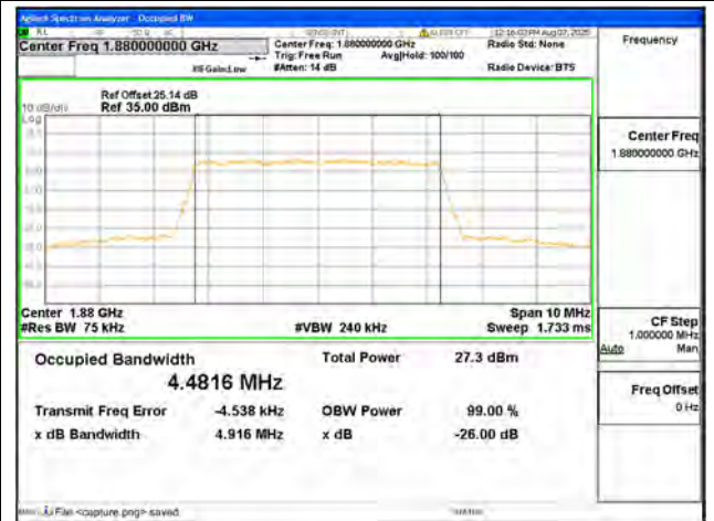
B2 / 5MHz / 16QAM/ Mid CH
