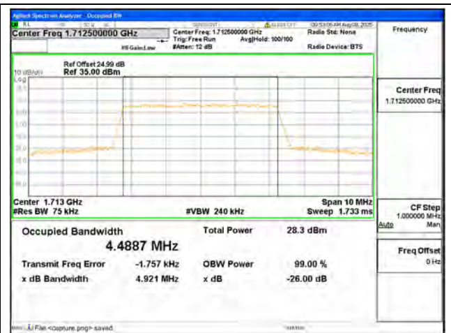
B4 / 5MHz / 16QAM/ Low CH
