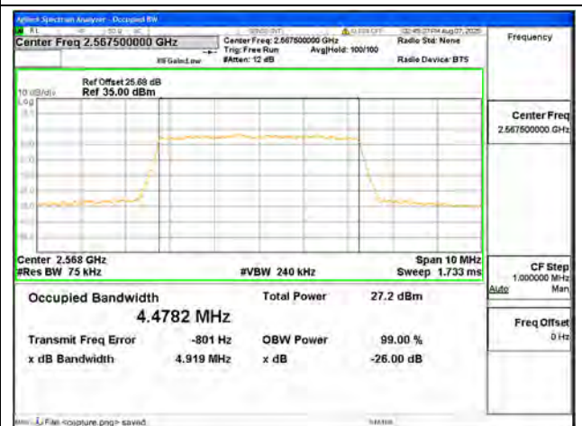
B7 / 5MHz / 16QAM/ High CH
