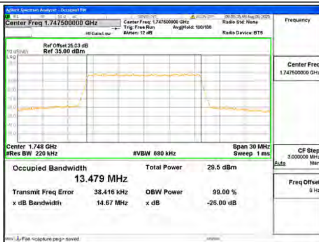
B4 / 15MHz / QPSK/ High CH
