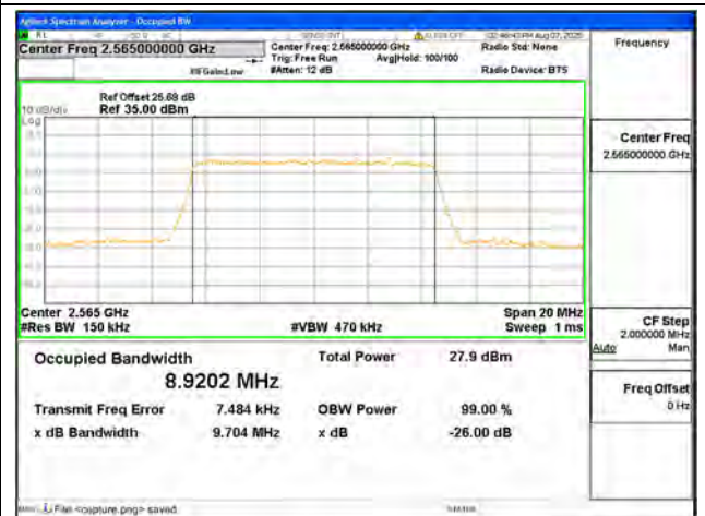
B7 / 10MHz / 16QAM/ High CH
