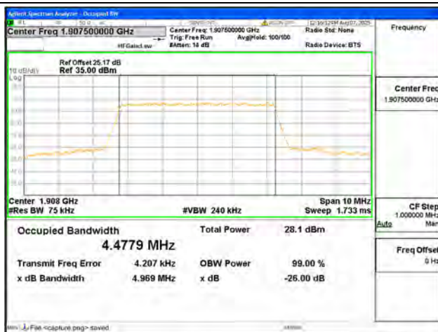
B2 / 5MHz / QPSK/ High CH
