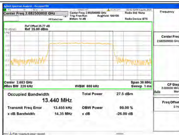
B41 / 15MHz / QPSK/ High CH
