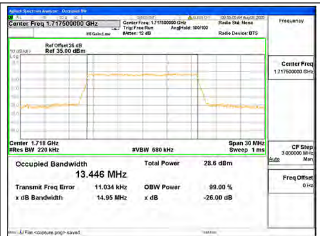
B4 / 15MHz / 16QAM/ Low CH
