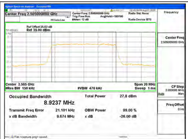
B7 / 10MHz / 16QAM/ Low CH
