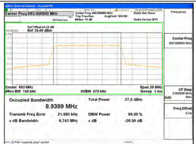
B71 / 10MHz / 16QAM/ High CH
