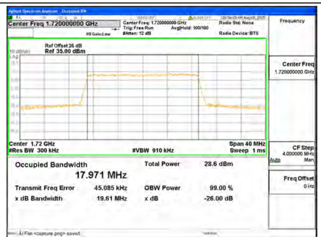
B4 / 20MHz / 16QAM/ Low CH
