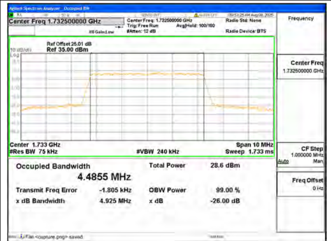
B4 / 5MHz / 16QAM/ Mid CH
