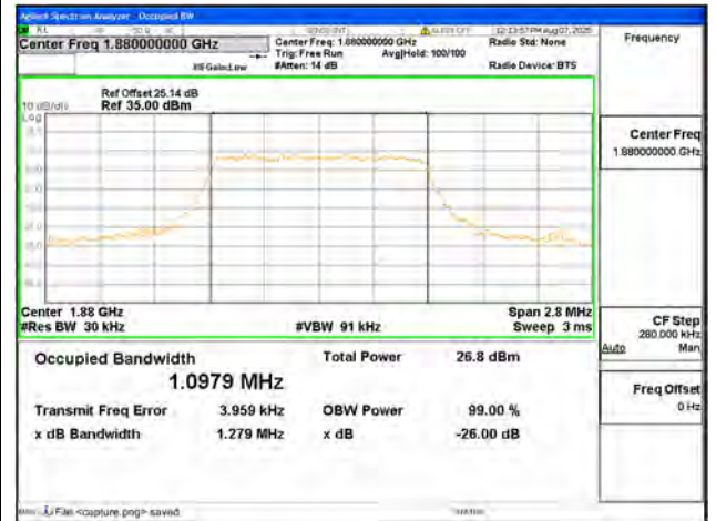
B2 / 1.4MHz / 16QAM/ Mid CH
