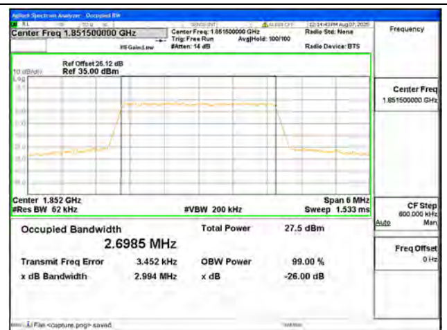
B2 / 3MHz / 16QAM/ Low CH
