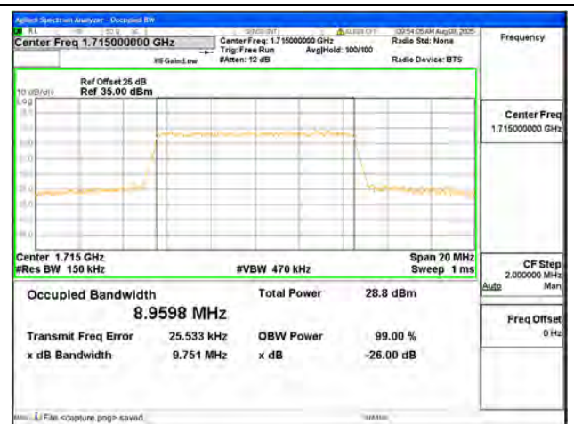
B4 / 10MHz / 16QAM/ Low CH
