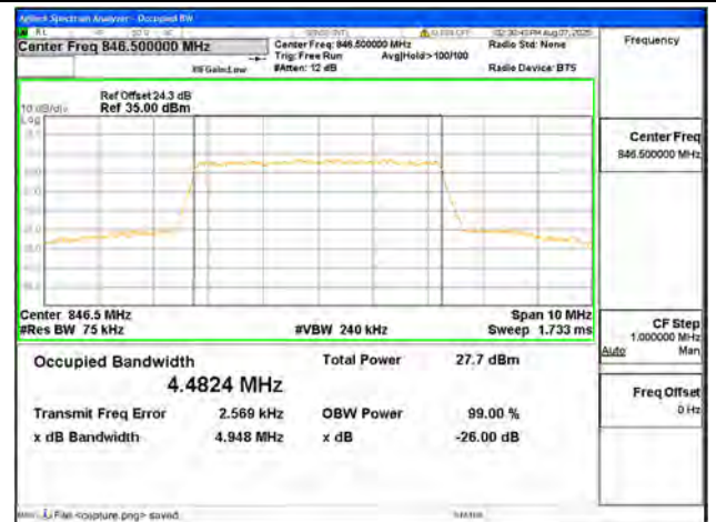
B5 / 5MHz / 16QAM/ High CH
