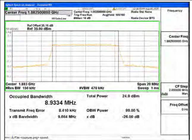
B25 / 10MHz / 16QAM/ Mid CH
