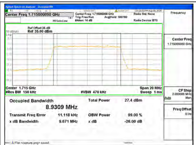
B66 / 10MHz / 16QAM/ Low CH
