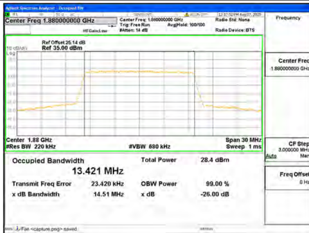
B2 / 15MHz / QPSK/ Mid CH
