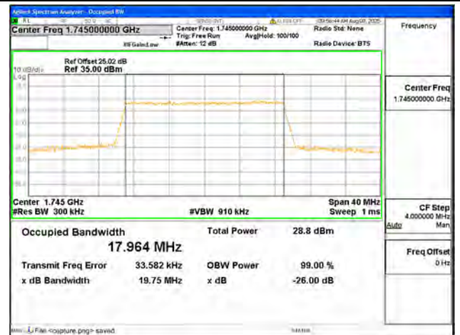
B4 / 20MHz / 16QAM/ High CH
