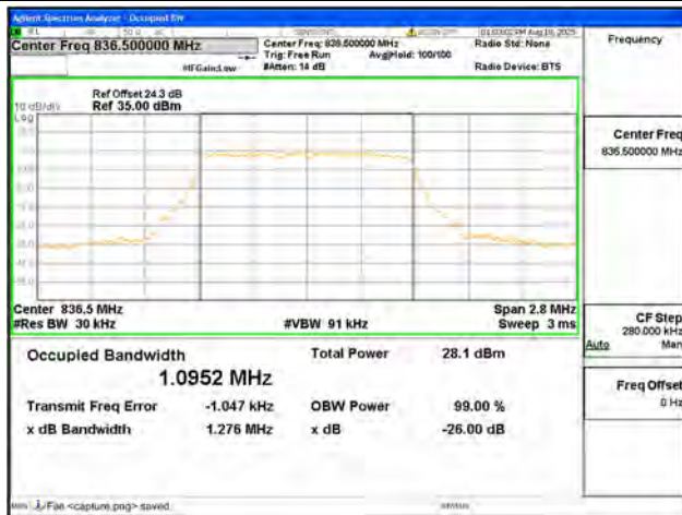
B26 Part22 / 1.4MHz / QPSK/ Mid CH
