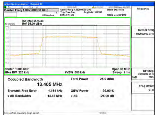
B25 / 15MHz / 16QAM/ Mid CH
