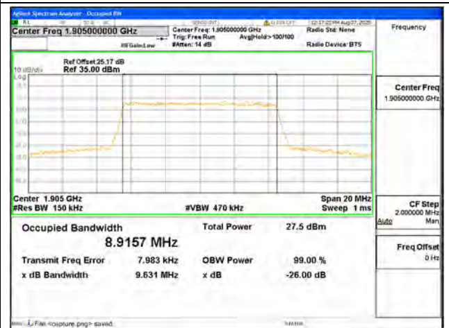
B2 / 10MHz / 16QAM/ High CH
