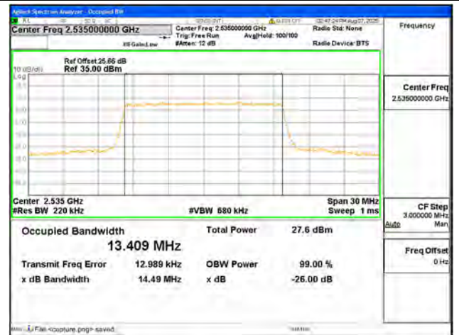
B7 / 15MHz / 16QAM/ Mid CH
