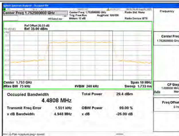
B4 / 5MHz / QPSK/ High CH
