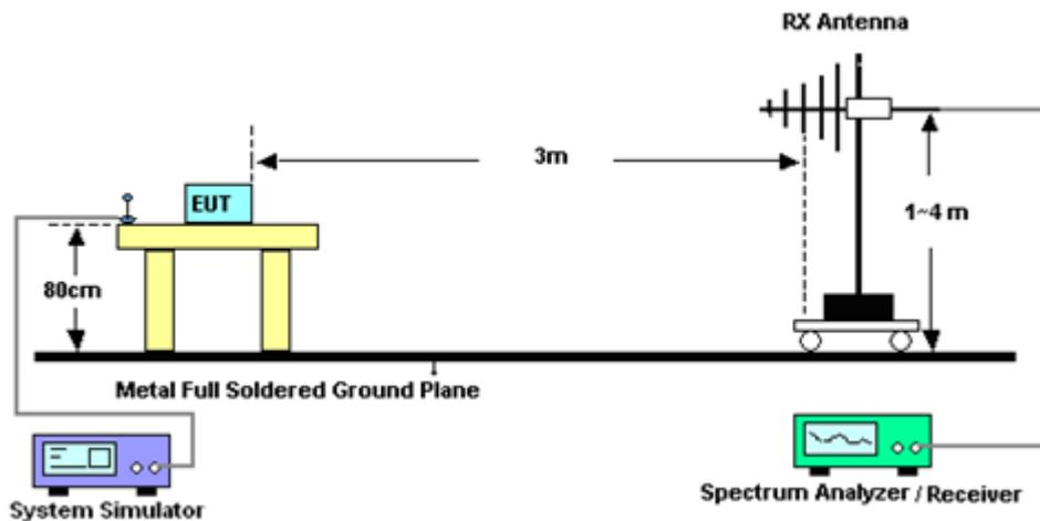
For radiated test from 1GHz to 18GHz
