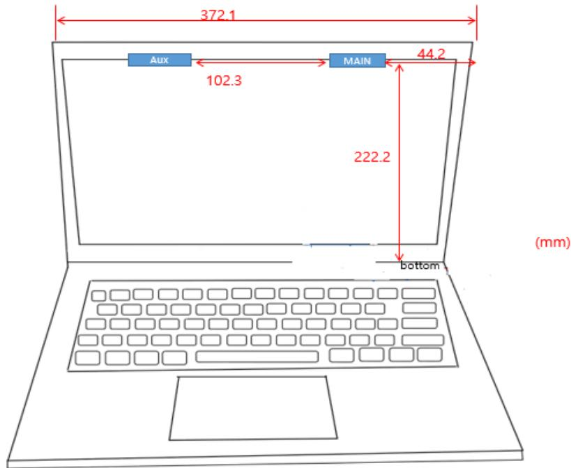
The antenna of this product, under normal use condition, is at least 20 cm away from bottom. So, this device is classified as Mobile device.
