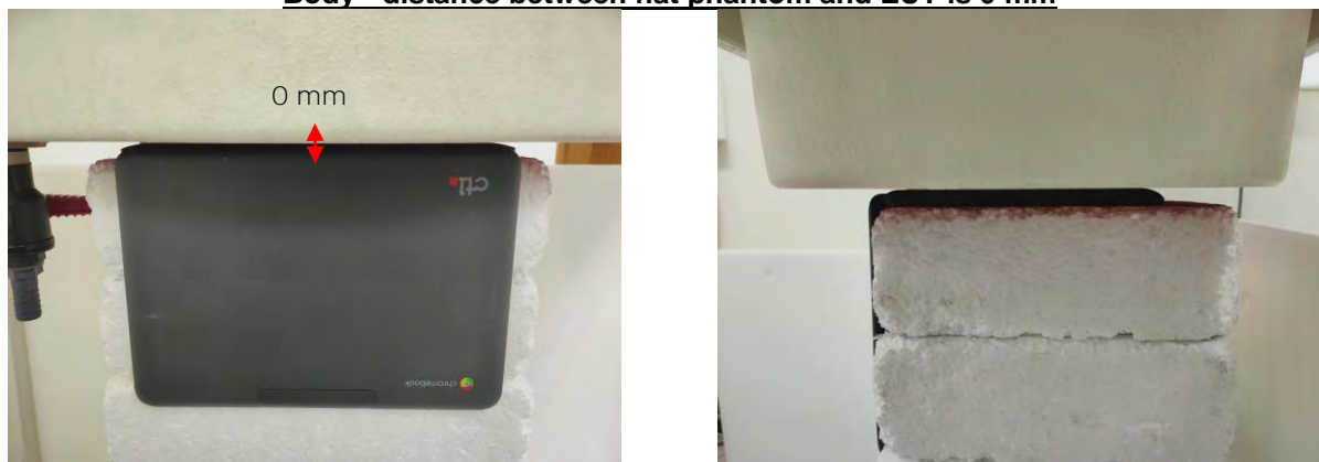
Fig.3 EUT Bottom side to flat phantom
