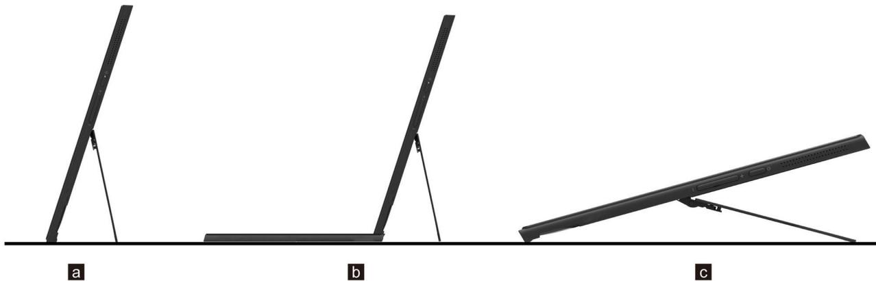
The kickstand is multi-positional. You can adjust the kickstand to various angles for a comfortable user experience.
