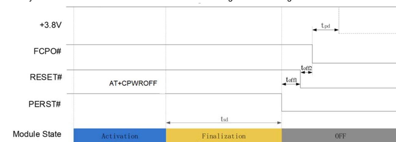
Figure 3-6 Software control power off timing
