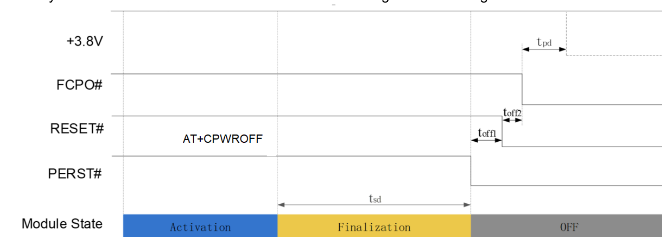
Figure 3-6 Software control power off timing
