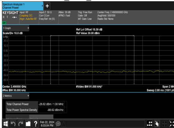
N41(20M)_DFT-s-OFDM_QPSK_Outer_Full_Low_CH CHP PASS
