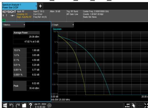
N77(20M)_DFT-s-OFDM_PI_2- BPSK Outer Full Mid CH
