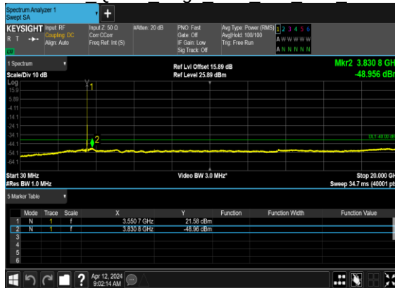
N48(10M)_DFT-s- OFDM QPSK Edge 1RB Left Low CH
