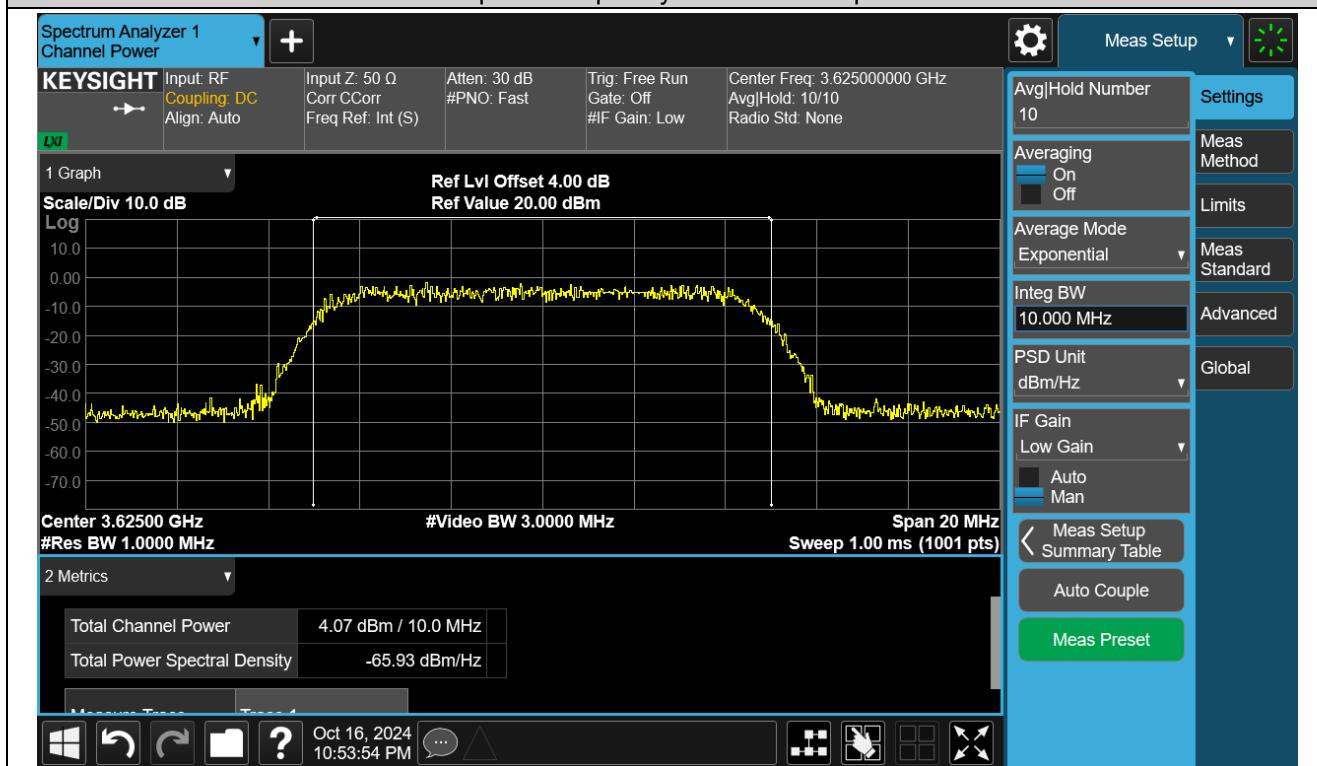
EUT stops transmission within 10 seconds of receiving instructions from its associated CBSD.
