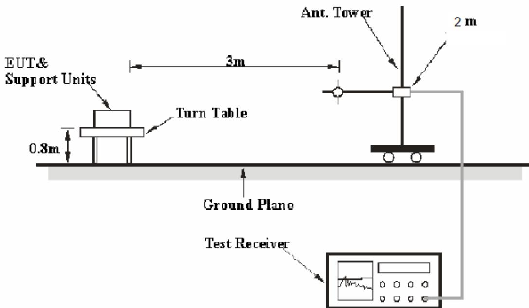
The radiated emission tests were performed in the 3 meters chamber test site, using the setup accordance with the FCC MP - 5.
