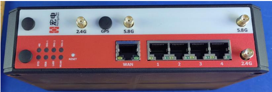
Figure2-1 Physical drawing of the appearance of the MRR8860 industrial intelligent gateway
