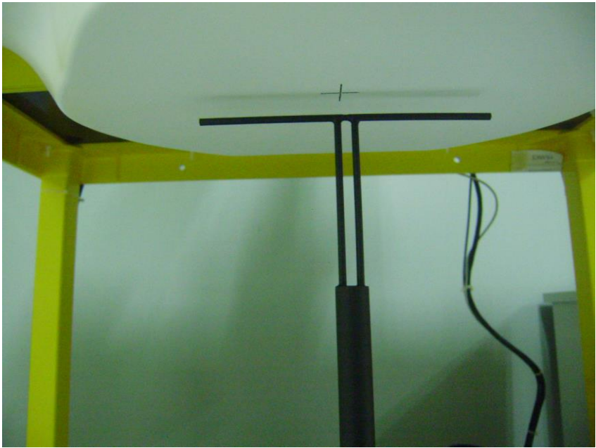
Setup Photo of Dipole Antenna
