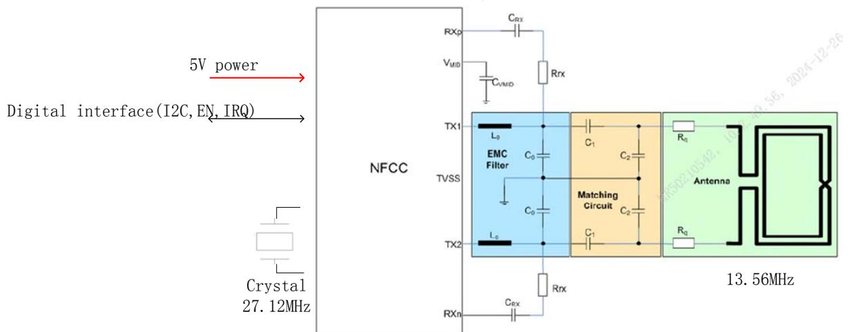
This NFC module can work in two Work Mode modes:
