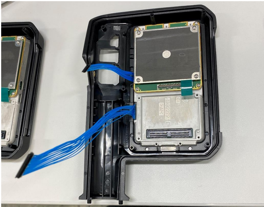
Figur 28 Diversity antenna and cables mounted mounted
