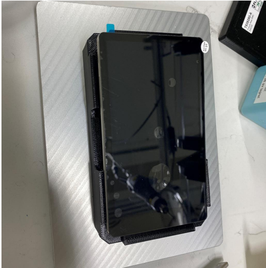
Figur 34 Screen glued in place
