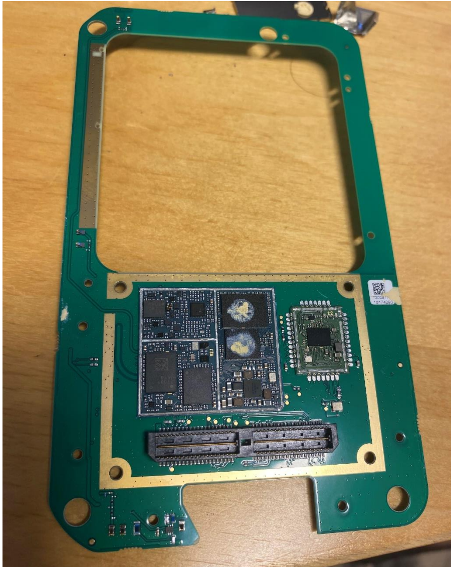
Figur 21 ETRA without radio module covers
