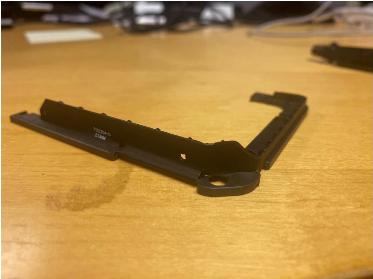
Figur 13 Antenna LTE main
