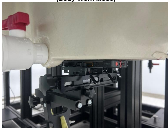
Rear Face of EUT with 0 cm Gap (Extremity Mode)
