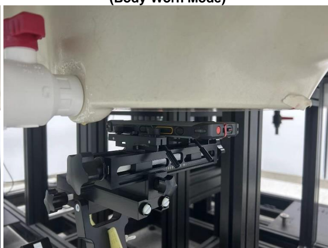
Rear Face of EUT with 1.4 cm Gap (Body-Worn Mode)
