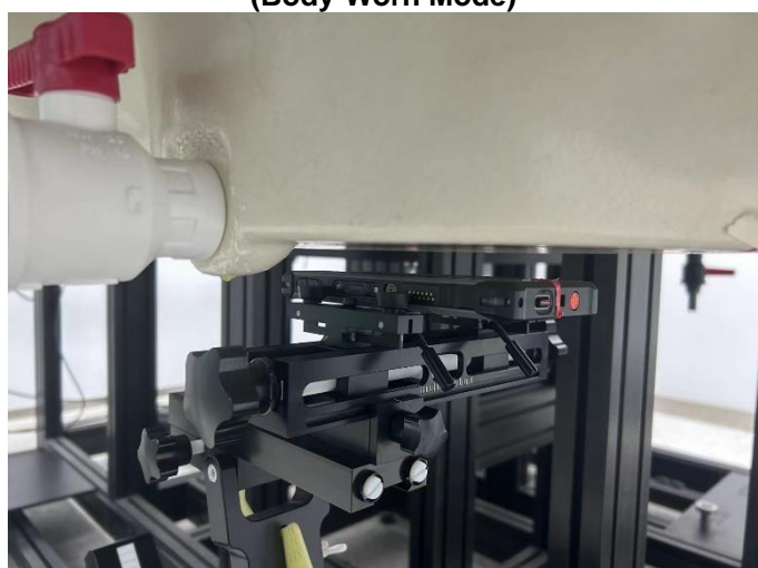
Front Face of EUT with 1.4 cm Gap (Body-Worn Mode)
