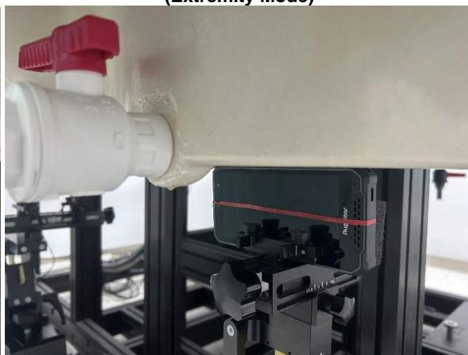
Right Side of EUT with 0 cm Gap (Extremity Mode)
