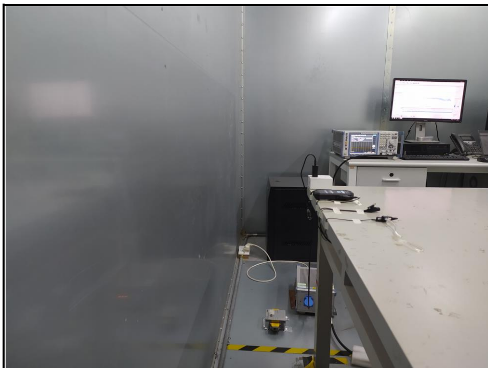
Fig. 3 Power line conducted emission setup photo
