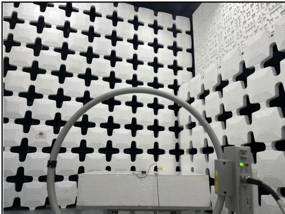
Fig. 1 Radiated emission setup photo(Below 30MHz)
