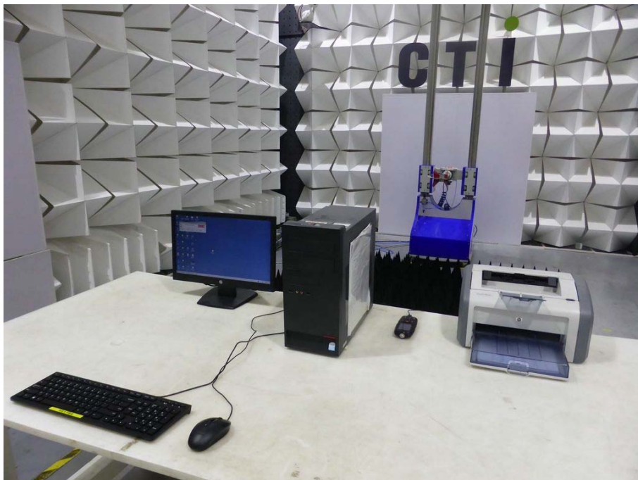
Radiated emission Test Setup-1 (Above 1GHz)
