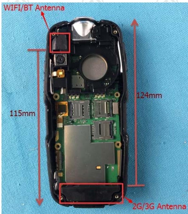
The SAR measurement positions of each side are as below:
