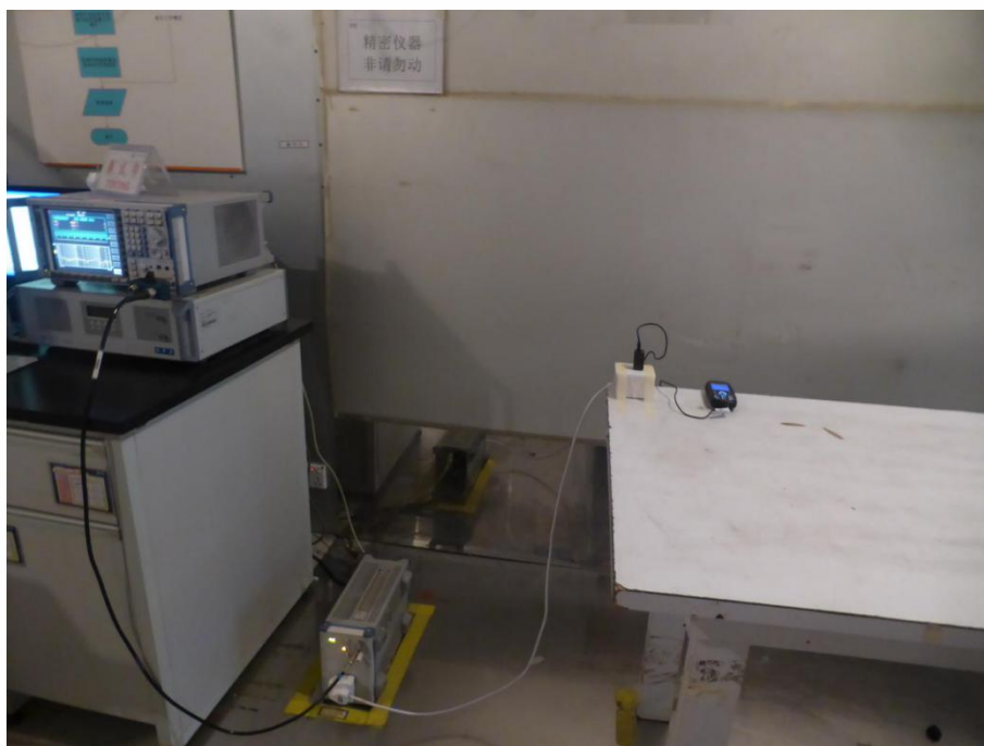
Conducted Emissions Test Setup
