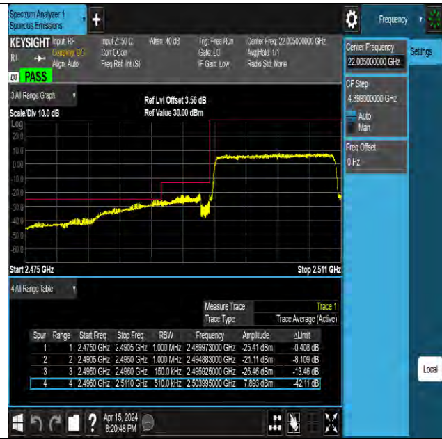
Band41 15MHz QPSK 39725 75RB#0
