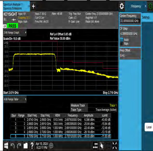
Band41 15MHz 16QAM 41515 75RB#0
