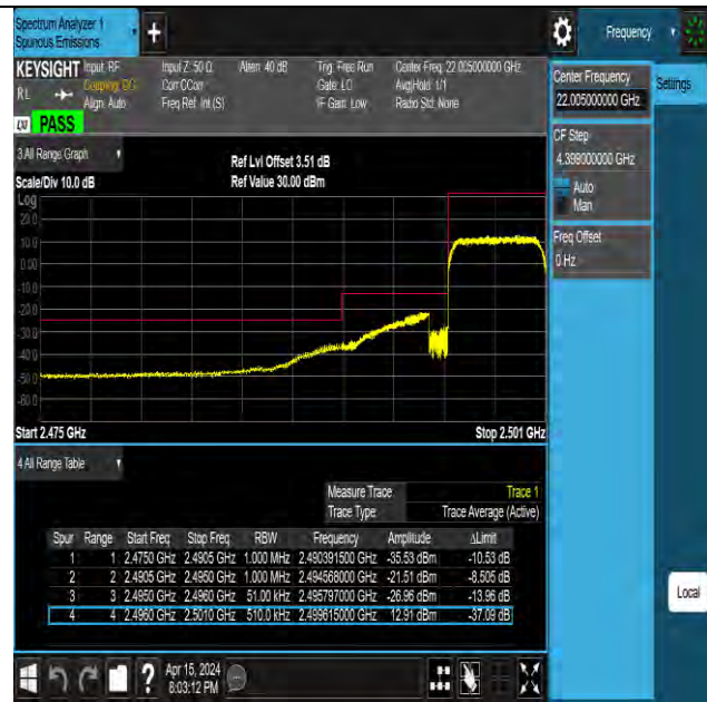
Band41 5MHz QPSK 39675 25RB#0
