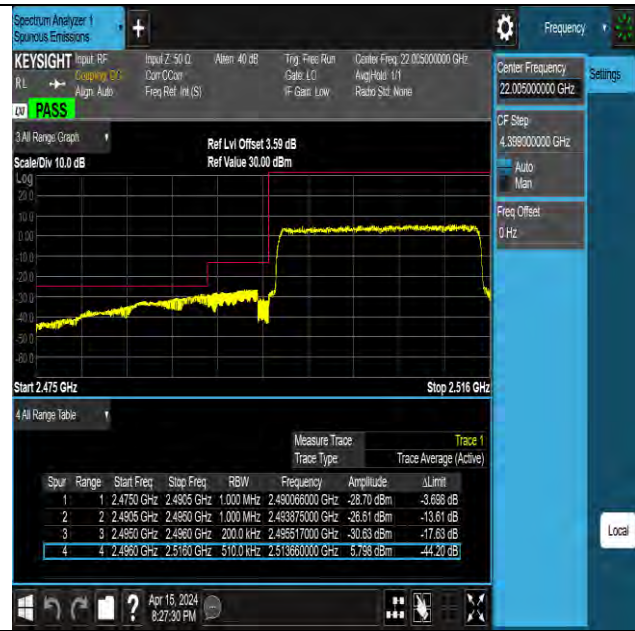
Band41 20MHz 16QAM 39750 100RB#0
