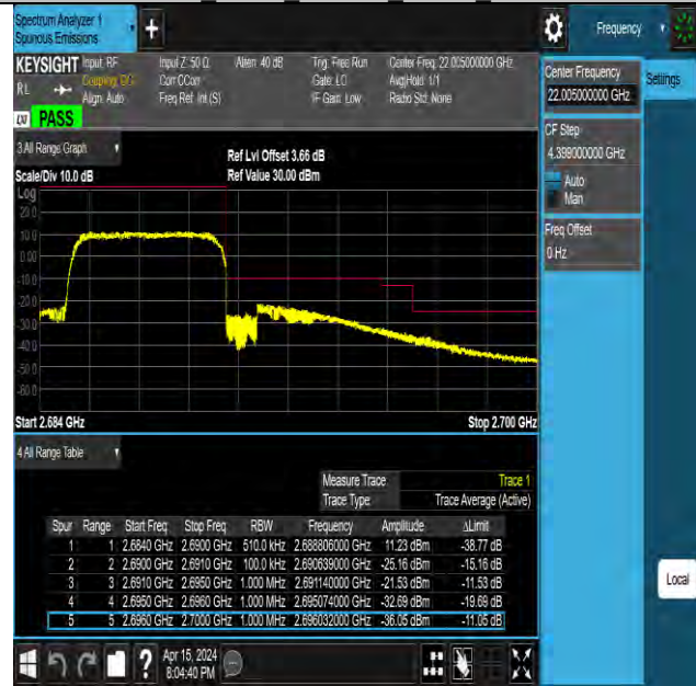
Band41 5MHz 16QAM 41565 25RB#0
