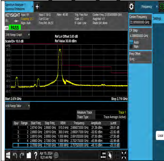
Band41 15MHz 16QAM 41515 1RB#74
