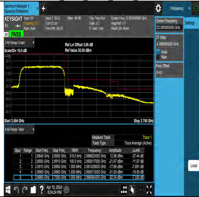
Band41 5MHz QPSK 41565 25RB#0
