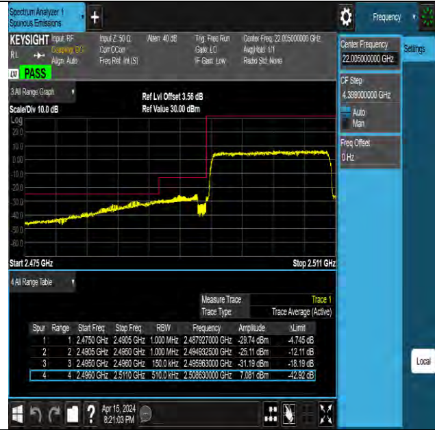
Band41 15MHz 16QAM 39725 75RB#0
