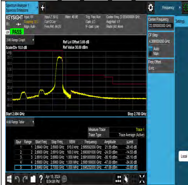
Band41 5MHz 16QAM 41565 1RB#24
