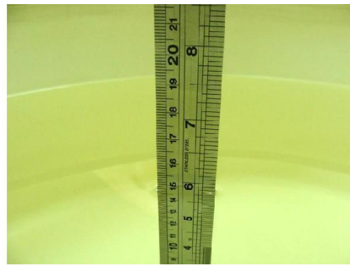
Fig 7.2 Photo of Liquid Height for Body SAR
