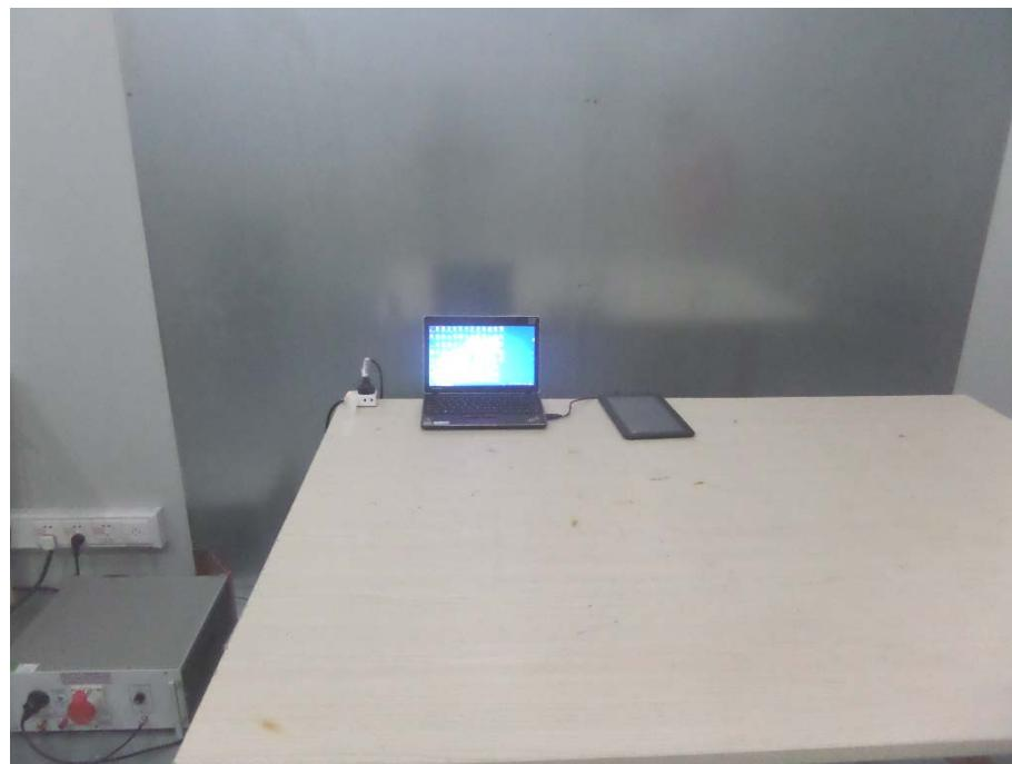
**Radiation Emission Test Setup (Below 30MHzz)***Charging & playing mode*
