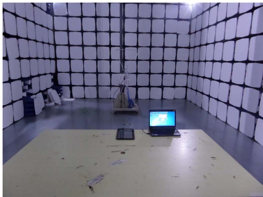
**Radiation Emission Test Setup (Above 1GHz)***Charging & Playing Mode*
