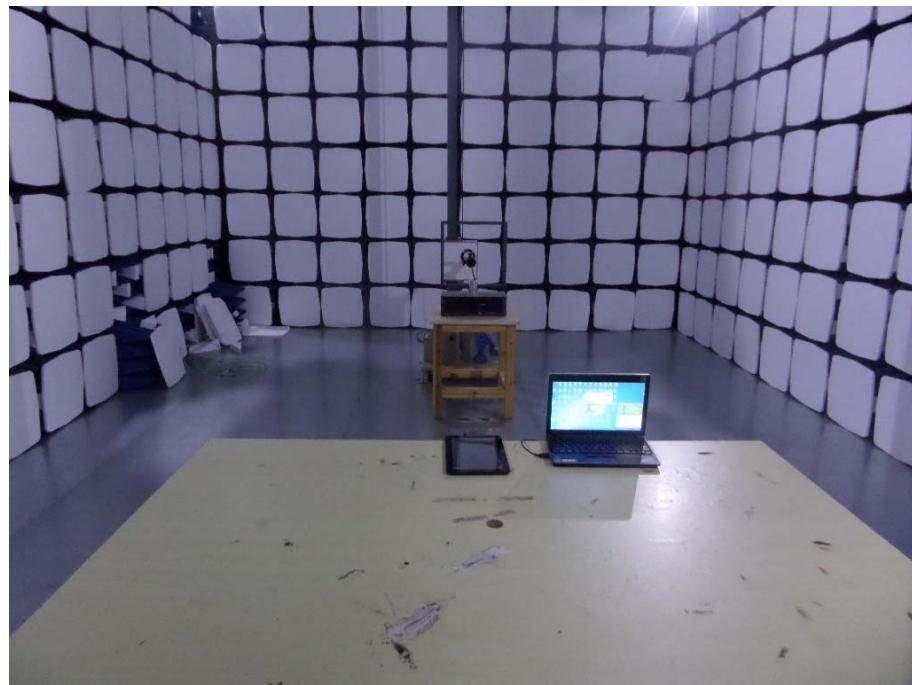
**Radiation Emission Test Setup (Below 30MHz to 1GHz)***Charging & Playing Mode*
