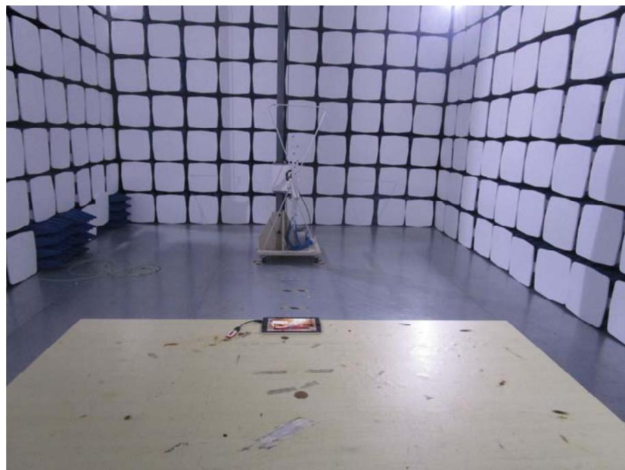
**Radiation Emission Test Setup (Above 1GHz)***Charging & Playing & Camera Mode*
