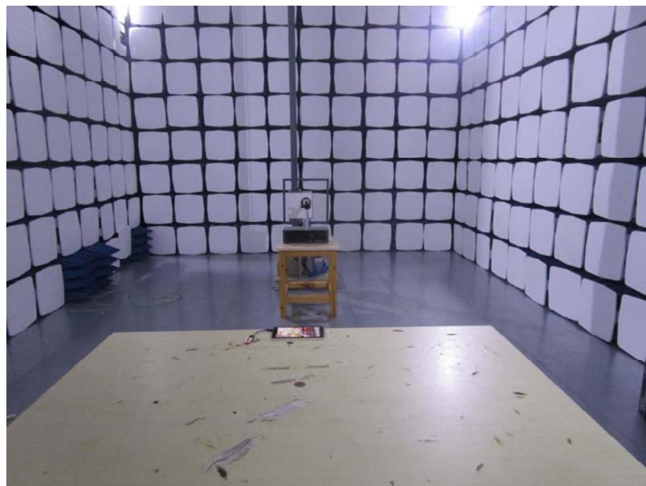
**Radiation Emission Test Setup (30MHz to 1GHz)***Charging & Playing & Camera Mode*
