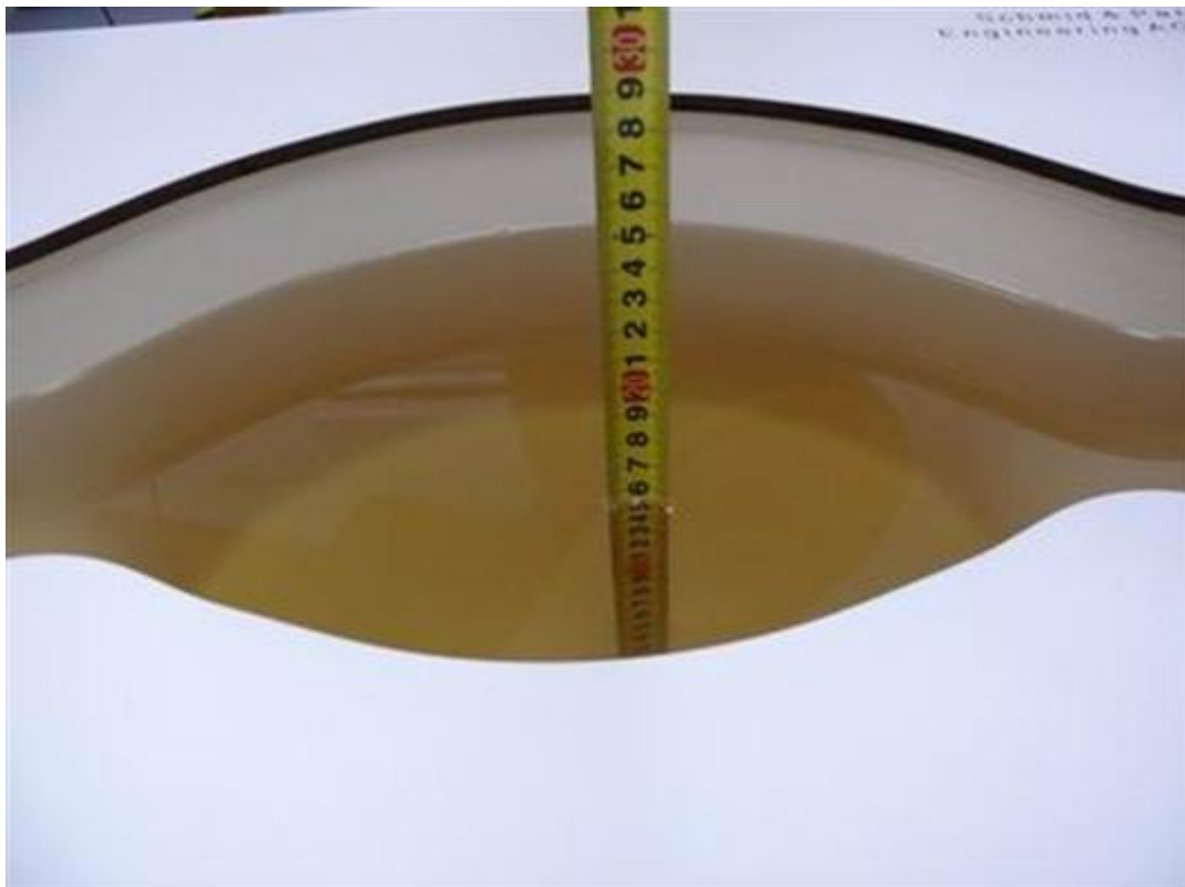
Picture 2: Liquid depth in the Flat Phantom (450 MHz, 15.4cm depth)
