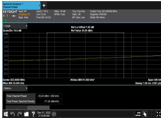
N5(20M)_DFT-s- OFDM_QPSK_Edge_1RB_Left_Low_CH_CHP_PA SS
