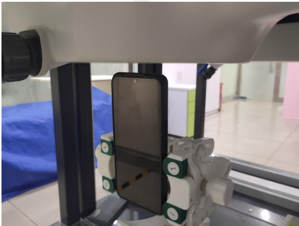
Body Top side(separation distance is 10mm)
