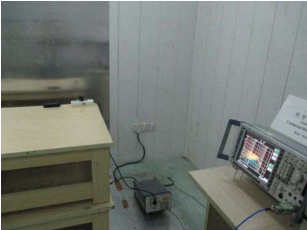
FCC RADIATED EMISSION TEST SETUP
