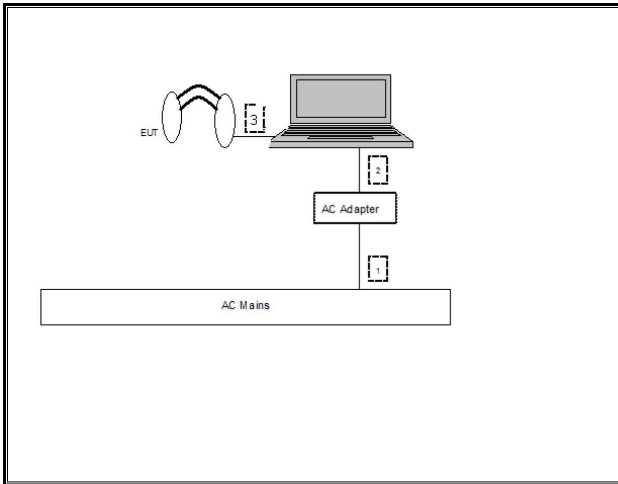
**FOR BELOW 1G RADIATED AND LC TEST SETUP**
