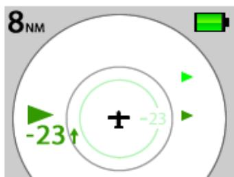
*Aircraft in the vicinity are displayed as green arrows of different size. The nearest aircraft not equipped with ADS-B or FLARM is indicated as a light green circle.*
