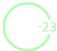
Green circle: the green circle gives the position of the nearest aircraft not equipped with ADS-B or FLARM, i.e. aircraft with Mode-C/S transponders. The height information is given in 100 ft steps and the circle symbolises the distance. (Example: 2300ft lower)
