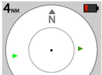
*When on the ground, the radar screen will operate provided there is adequate GPS reception. The screen image is always oriented to the north, symbolised in the screen by an 'N'.*
