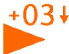
Large orange coloured arrow: this aircraft poses a threat of collision. The flight direction and height difference of the other aircraft are given to the nearest 100 ft,
