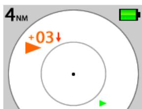
*In dangerous situations, aircraft posing a threat are presented in orange or red, depending on the urgency of the threat. An acoustic alarm is issued in addition to the optical alarm.*
