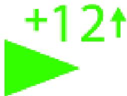
Large arrow with height information: the large arrow always indicates the nearest aircraft and its relative height in steps of 100 ft, together with climb/descent information. The arrow indicates the direction in which the target aircraft is flying above ground. For example: 2300ft lower, flying from left to right in a climb.
