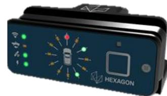
The LEDs on the left side of the display show the status of the system. They indicate if the device has enough power, has acceptable GNSS reception or is traveling backwards as well as other information about the system.
