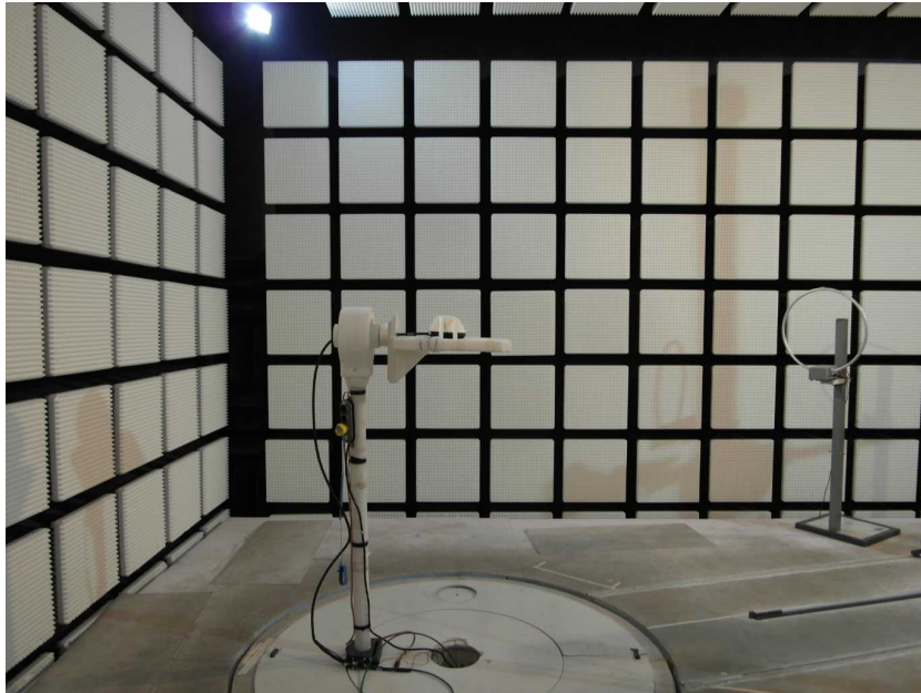
Photo 1: EUT at the anechoic chamber
