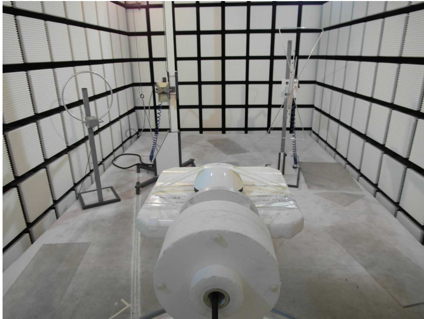
Photo 3: EUT at the anechoic chamber
