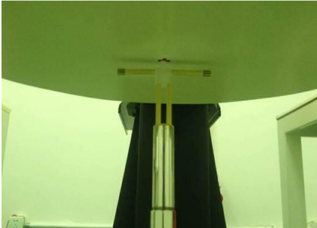
Picture 10-2 Photo of Dipole Setup
