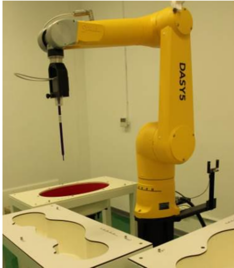
Picture 8-2: Specific Absorption Rate Test Layout
