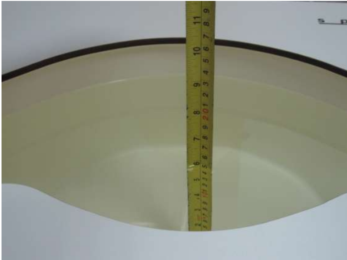
Picture C.3: Liquid depth in the flat Phantom (1900 MHz) (15.1cm deep)
