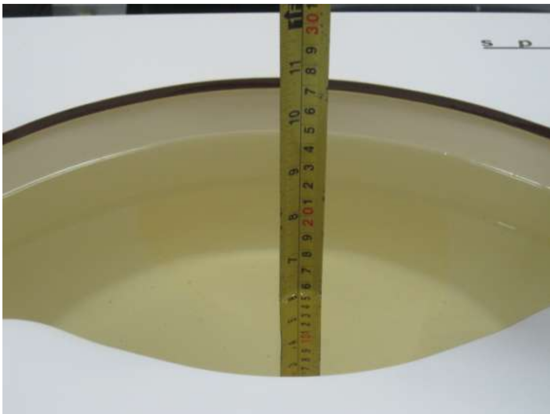
Picture C.2: Liquid depth in the flat Phantom (835MHz) (15.2cm deep)
