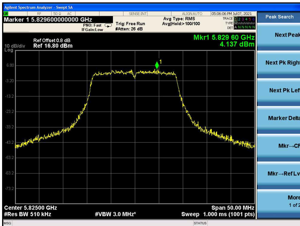
Fig.12 Power spectral density: CH165,11n
