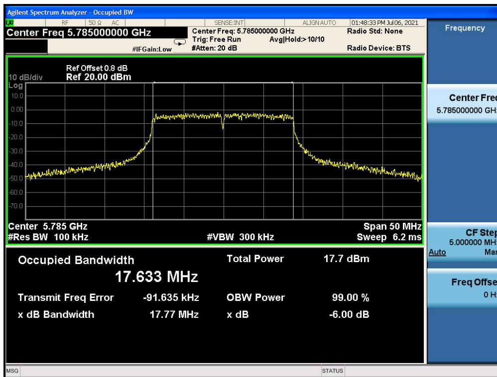
Fig.29 6dB Bandwidth: Ch157,11n
