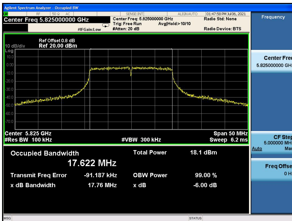
Fig.30 6dB Bandwidth: Ch165,11n
