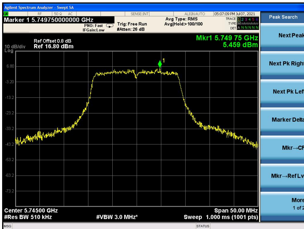
Fig.10 Power spectral density: CH149,11n
