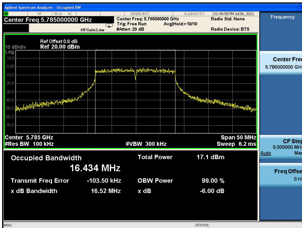
Fig.26 6dB Bandwidth: Ch157,11a
