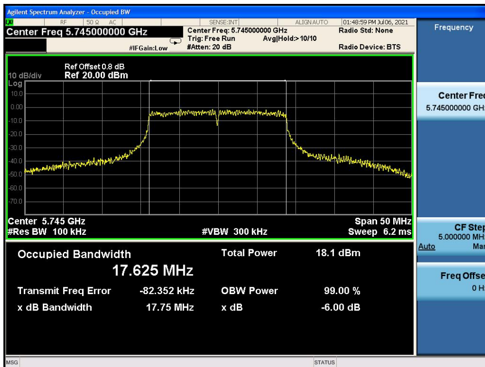
Fig.28 6dB Bandwidth: Ch149,11n
