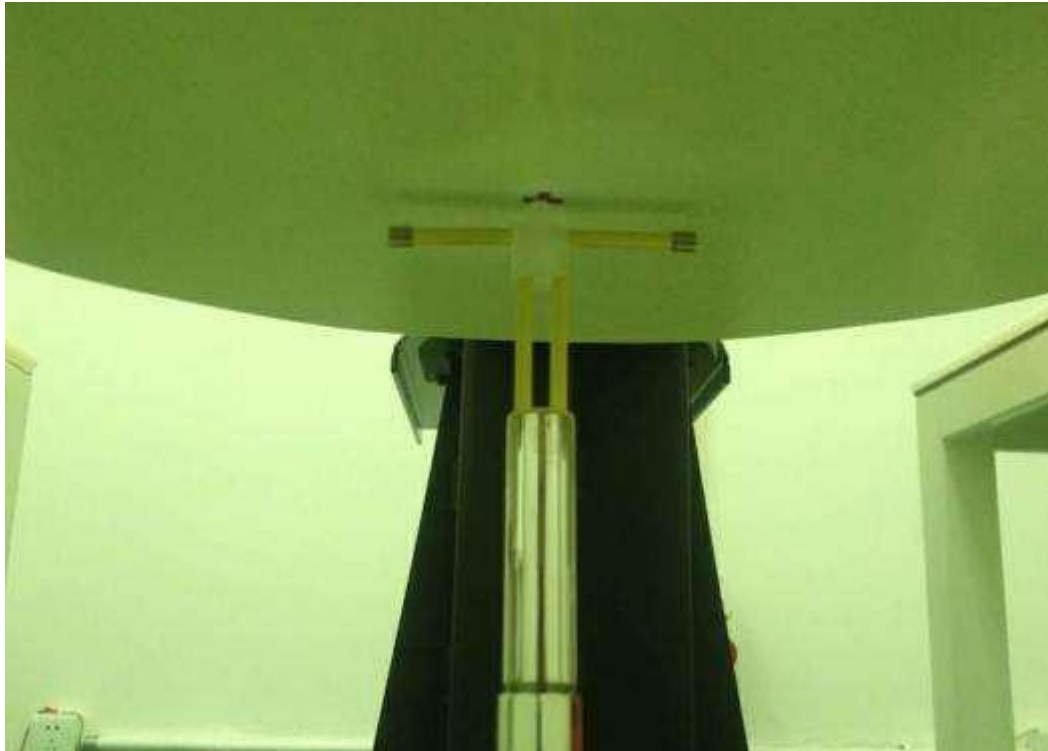
Picture 10-2 Photo of Dipole Setup
