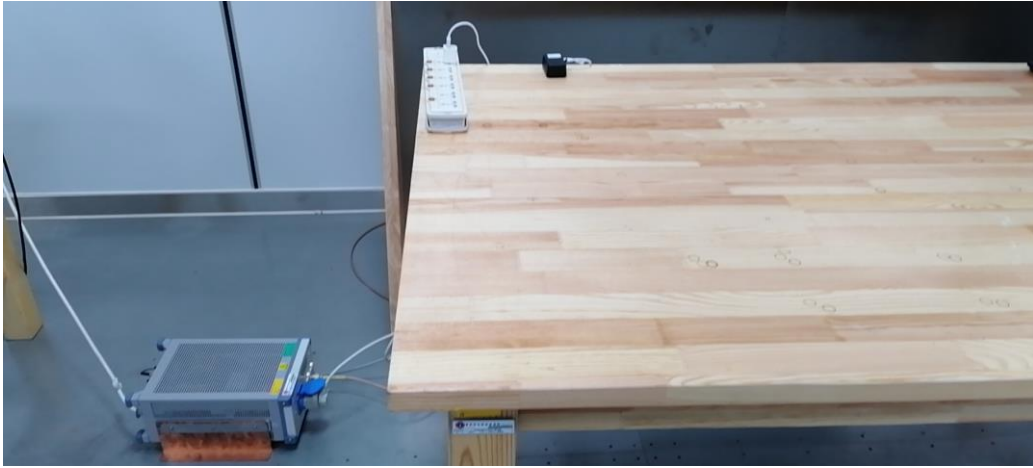
Pic3. Conducted (150KHz-30MHz)
