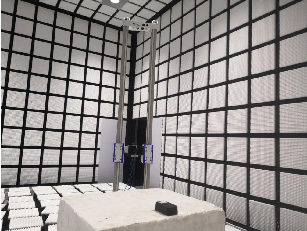
Pic2. Radiated emissions (1GHz-18GHz)
