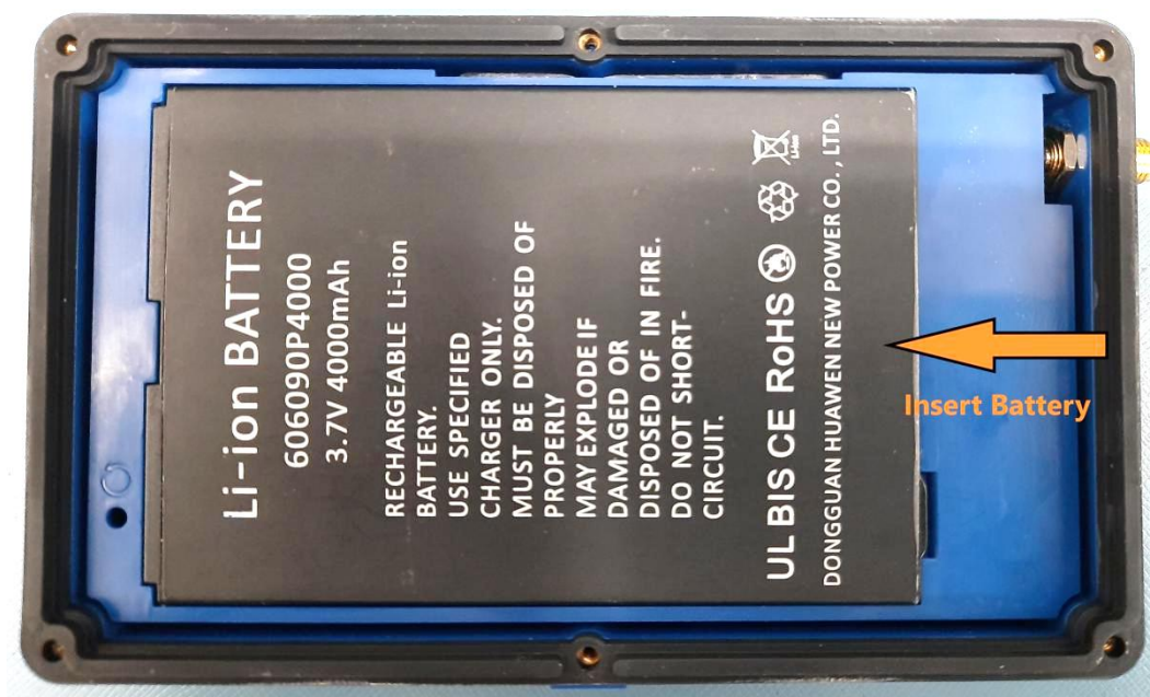
Figure 8 Insert battery in Mobile Hotspot unit, contacts facing downward.
