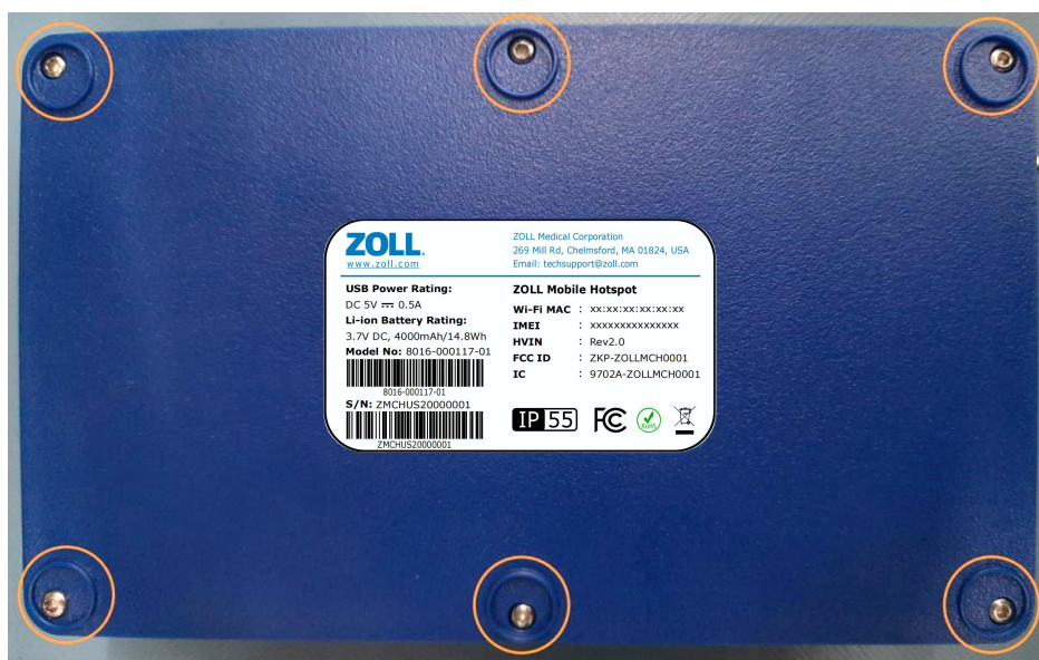
Figure 4 Turn the unit over & remove the six pads (marked in figure by Orange circles) to reveal the screws.
