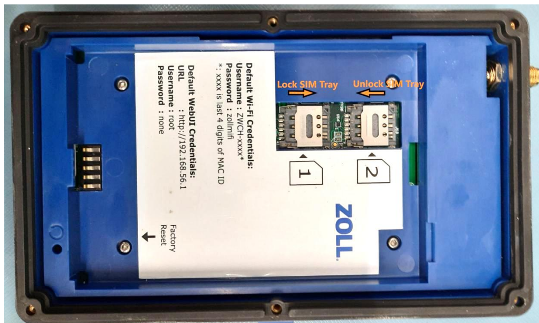
Figure 6 To insert the SIM card into the tray, unlock the tray by sliding the lock to the left, insert the SIM, and then slide the lock to the right to lock the SIM into place
