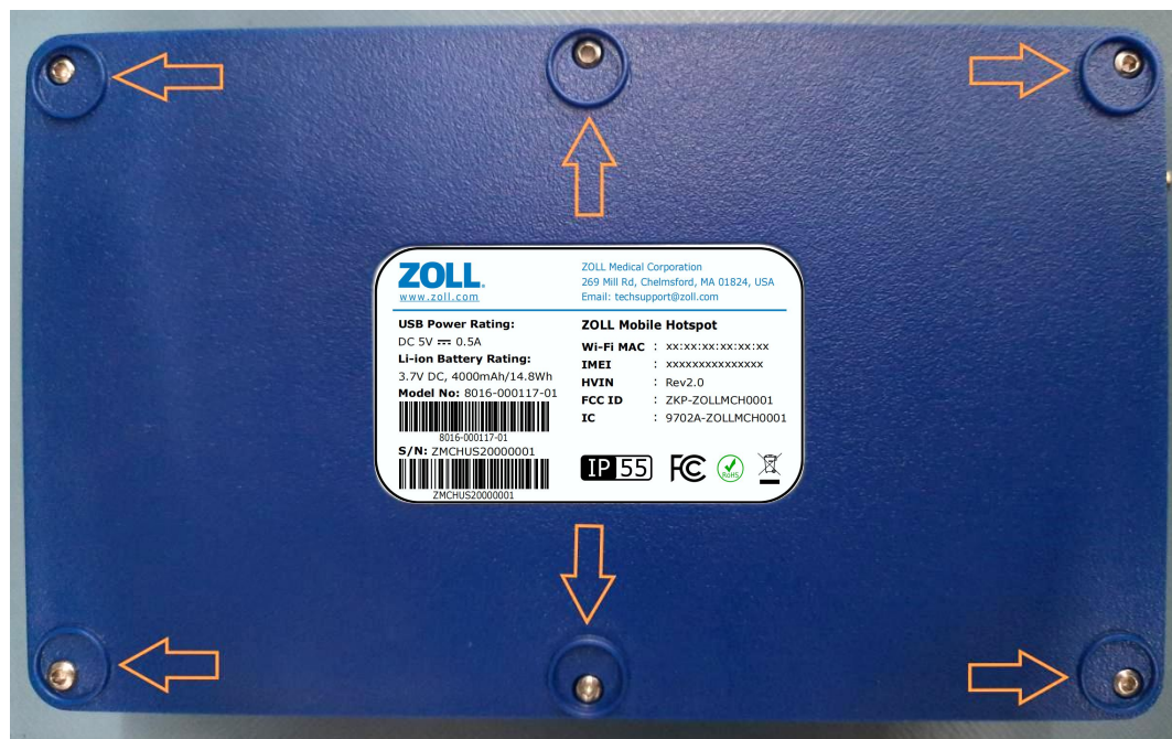
Figure 5 With screwdriver, remove the six screws.
