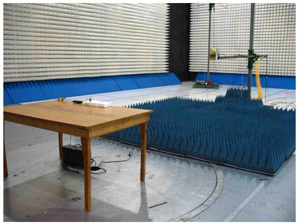
Radiated Emissions (Absorber in place for testing above 1GHz)
