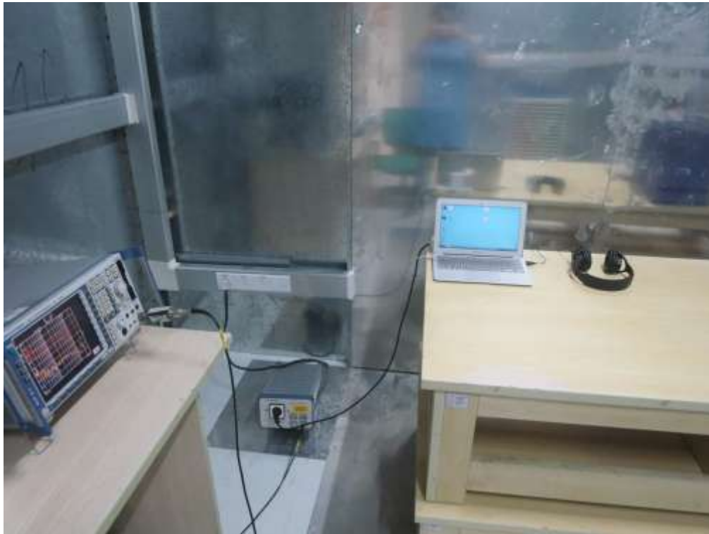
FCC RADIATED EMISSION TEST SETUP
