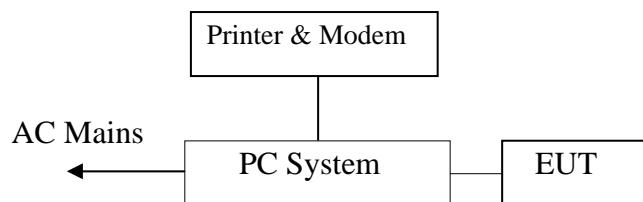
7.1.2. Semi-anechoic Chamber Test Setup Diagram
